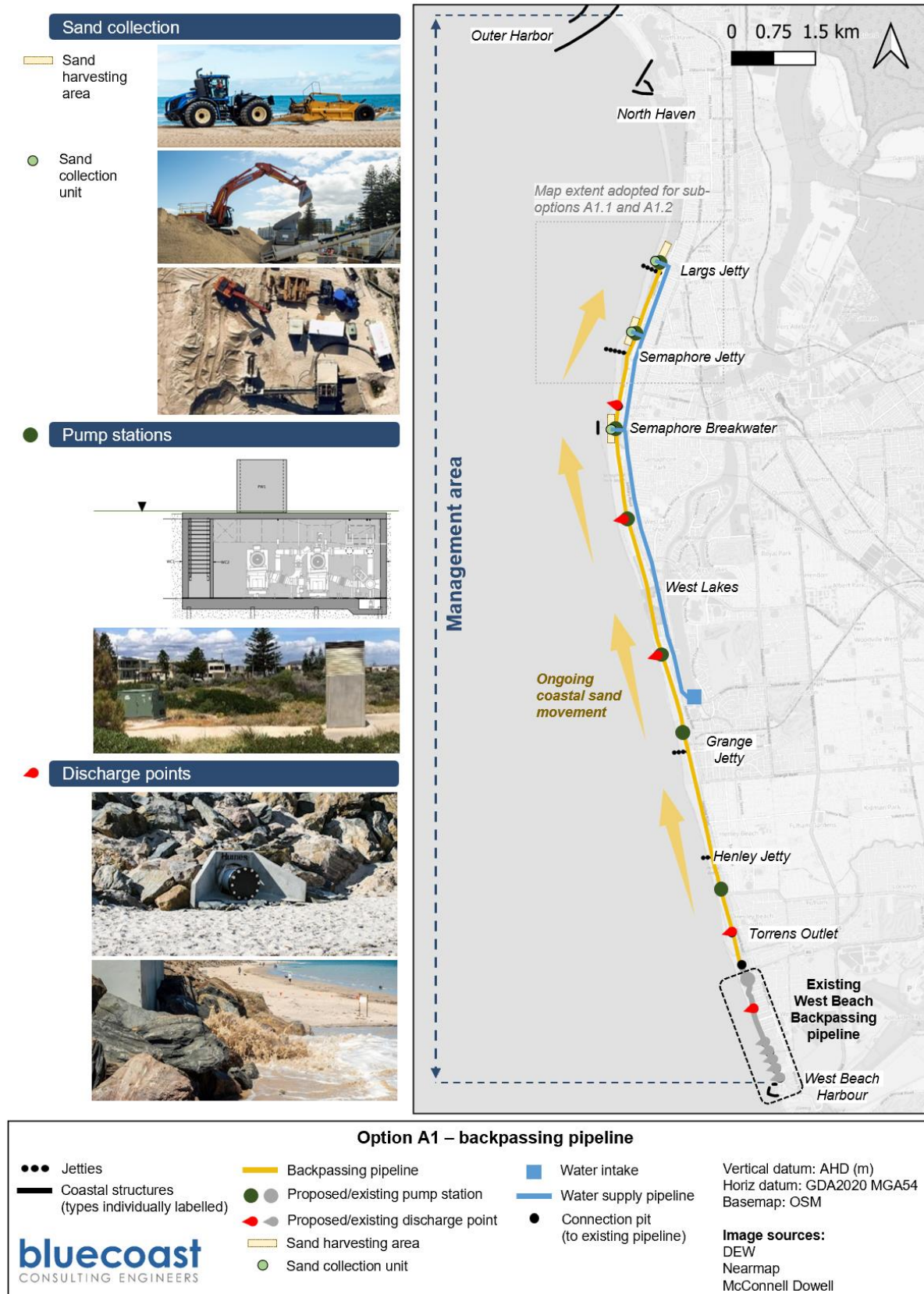
Figure 34: Conceptual design layout of the backpassing pipeline option (Option A1).
