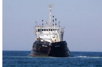
Split hopper TSHD, the David Allan, placing material as beneficial reuse for beach nourishment.
