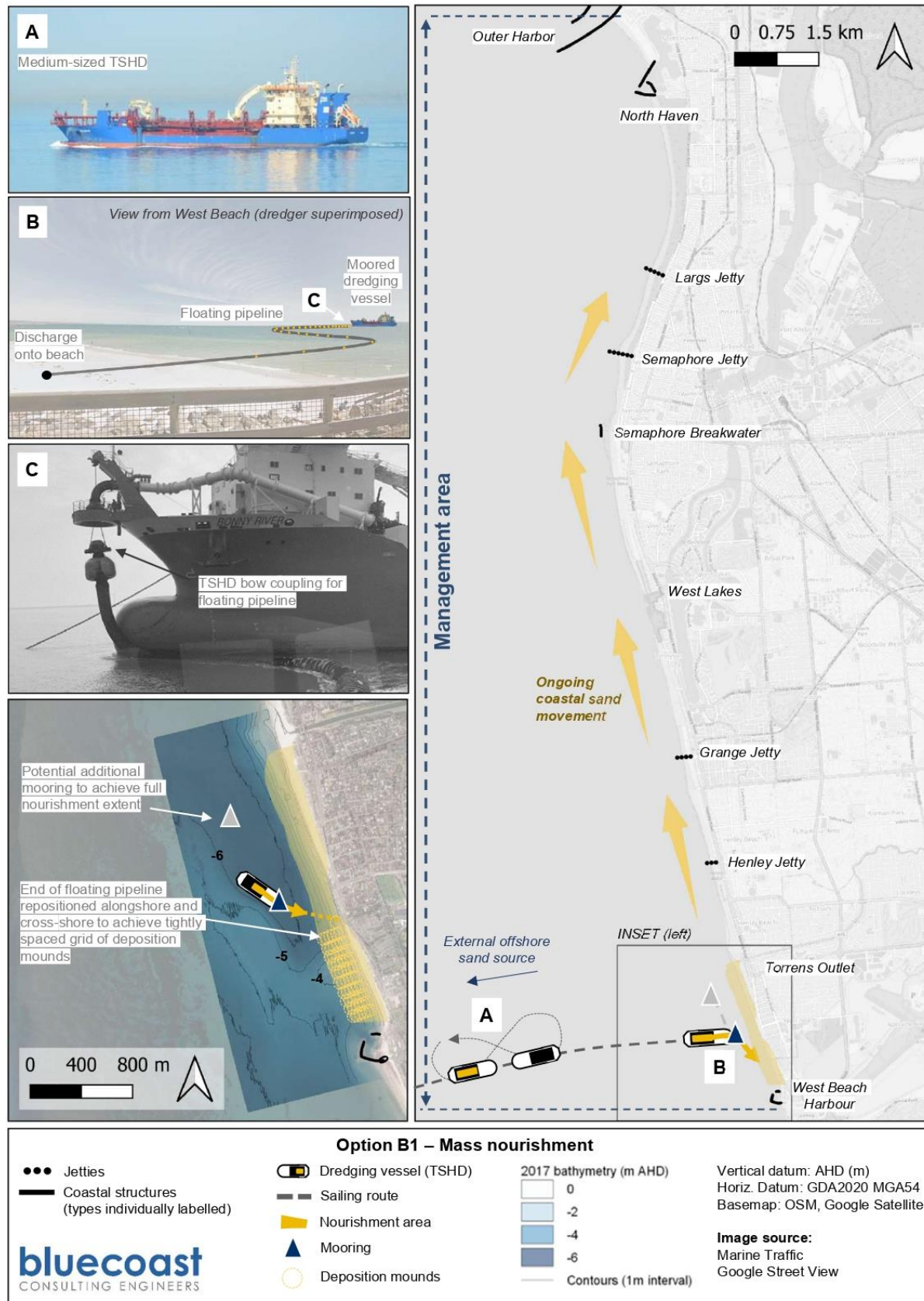
Figure 37: Conceptual design layout of the mass nourishment option (Option B1).
