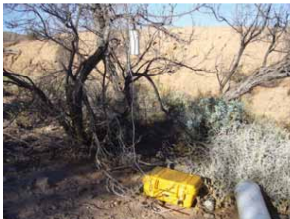
Figure 14. An Anabat kit (yellow box) with microphone in plastic tube (in bush) for recording bat calls (Photo: I. Williams).
