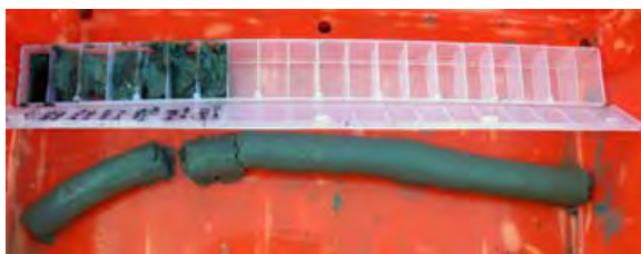
Extracted sample core, measured and sample layers placed in chip-tray with site number and depth recorded.
