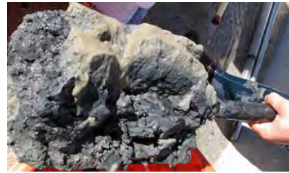
Soils being described, placed in chip-tray and mixed prior to placing in sample jars.
