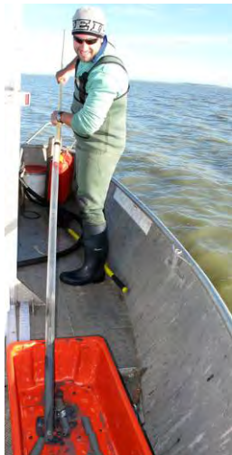
Sampling tube and suction used to obtain core samples in deeper water.
