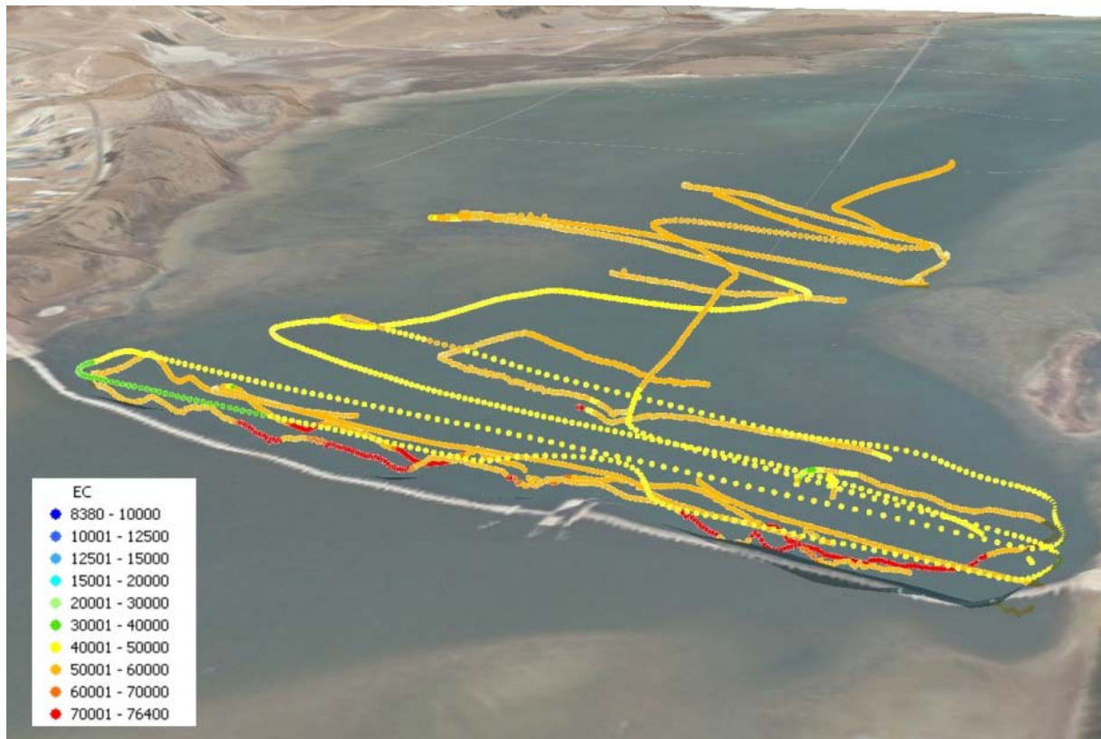
Figure 26: EC downstream of Goolwa barrage, January 2010
