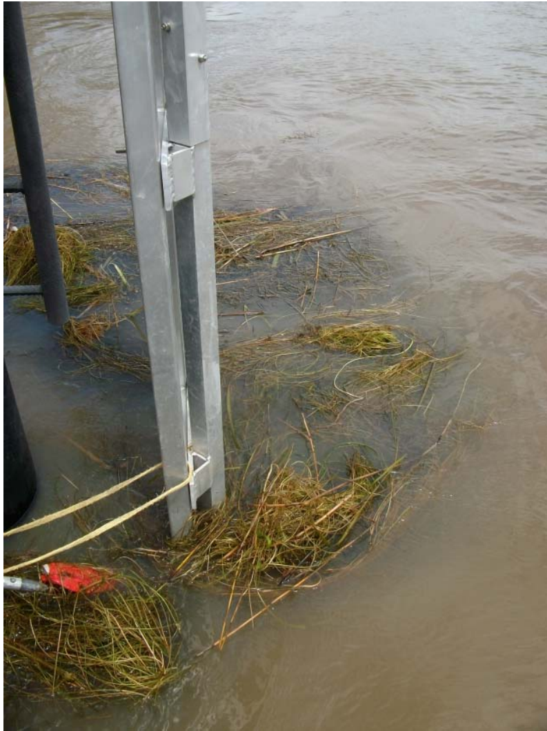
Figure 22 - Fouling of monitoring station
