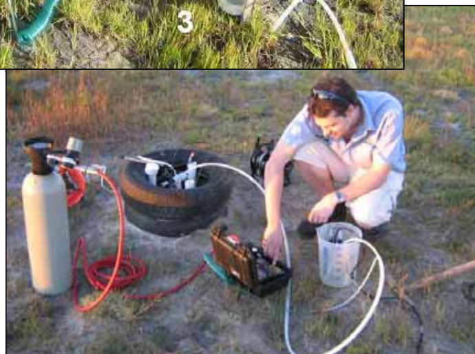
Plates 29-30. Above: All components of low-flow groundwater sampling kit: (1) Compressed CO 2 bottle; (2) QED MP10 controller; (3) Flow through cell for TPS water quality probe; (4) QED bladder pump; and (5) Steel cable for bladder pump and groundwater level sensor (for measurement of drawdown). Right: Low-flow sampling.
