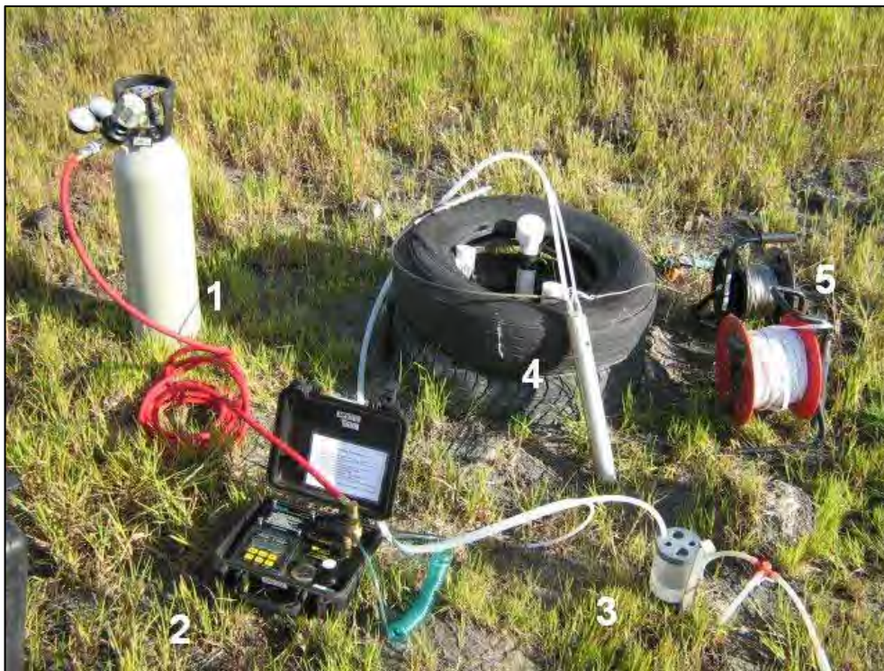
Plates 29-30. Above: All components of low-flow groundwater sampling kit: (1) Compressed CO 2 bottle; (2) QED MP10 controller; (3) Flow through cell for TPS water quality probe; (4) QED bladder pump; and (5) Steel cable for bladder pump and groundwater level sensor (for measurement of drawdown). Right: Low-flow sampling.
