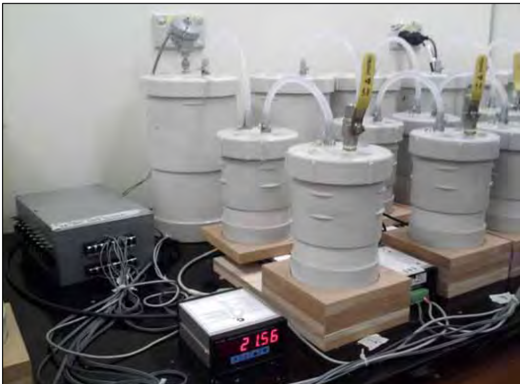
Plate 1. OxCon apparatus at CSIRO Land and Water laboratories, Urrbrae, SA. Shown mounted on load cell with adjacent power supply, data logger and temperature sensor.
