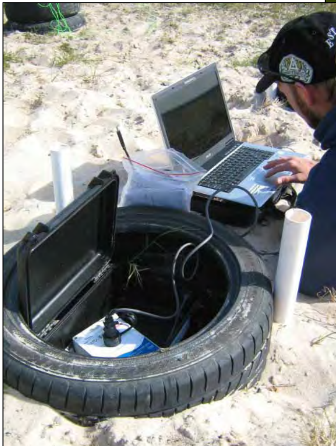
Plate 21. EnviroScan head unit with download port and power supply for moisture sensors and logging facility. Sediment moisture data is collected at 1 hour intervals in 10 cm depth intervals at the Point Sturt, Campbell Park and Windmill locations (see Figure 6).
