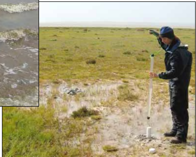
Plates 24-25. Collection of bulk groundwater samples for laboratory analysis.
