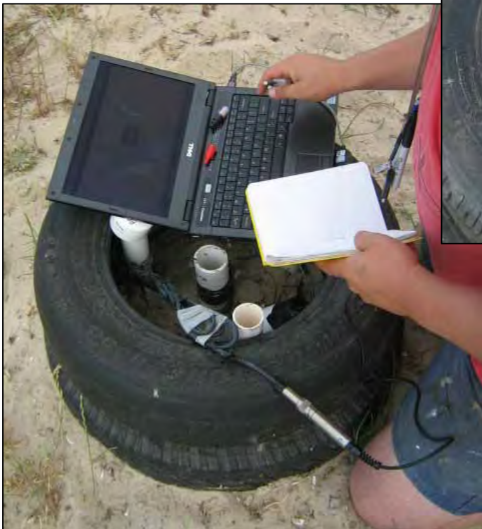
Plate 16. Data download from groundwater (piezometric) levels sensors.
