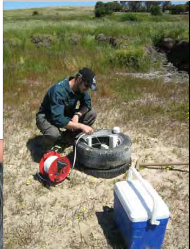
Plates 17-18. Verification of logged groundwater (piezometric) levels via manual dipping of piezometers.
