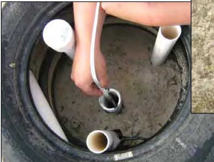
Plates 17-18. Verification of logged groundwater (piezometric) levels via manual dipping of piezometers.
