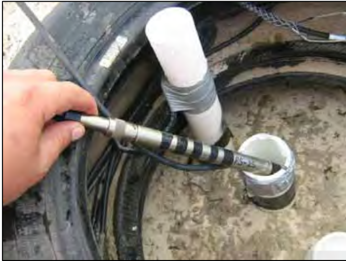
Plates 14-15. Installation of groundwater (piezometric) levels sensors.
