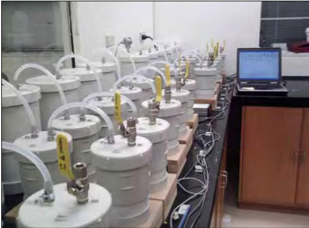
Plate 2. OxCon apparatus at CSIRO Land and Water laboratories, Urrbrae, SA. 12 of 14 apparatus shown with adjacent data logger, temperature and pressure sensors (top right of picture) and PC interface.
