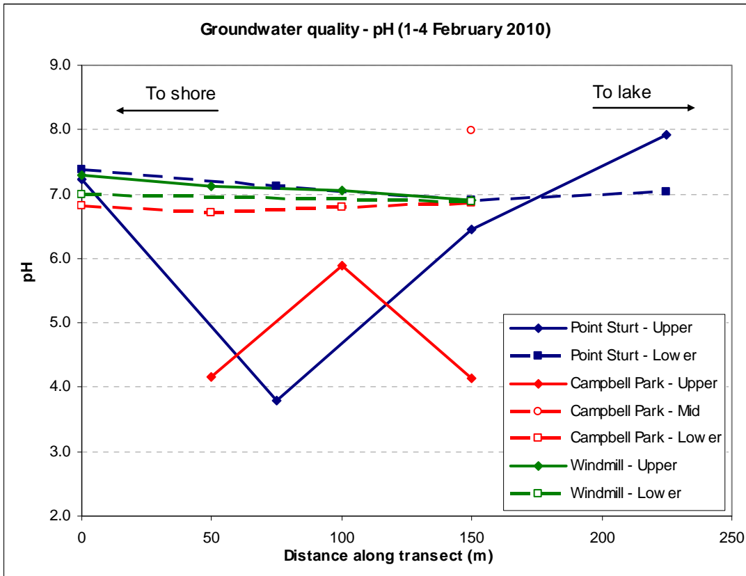
Figure 19. Groundwater pH at Point Sturt, Campbell Park and Windmill locations (after purging), 1-4 February 2010.
