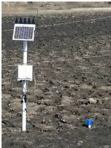
Figure 5 Sentek probe and telemetry station
