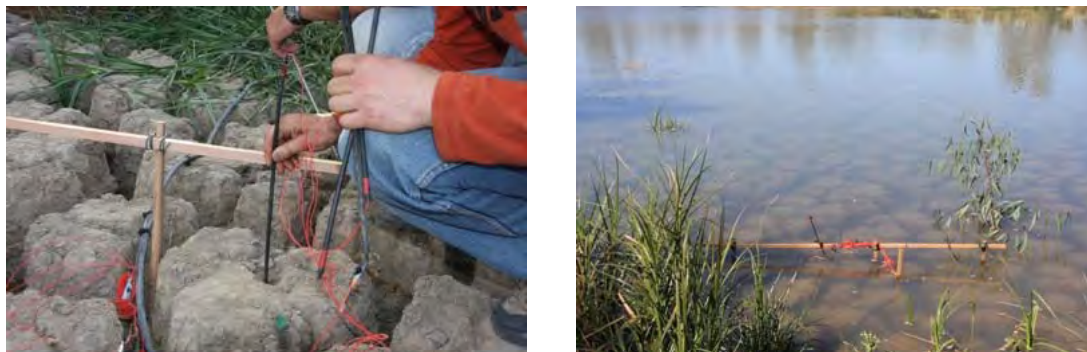
Figure 3 Installation of redox probes (Pt electrodes) in an SA wetland prior to rewetting (left) and following rewetting (right)
