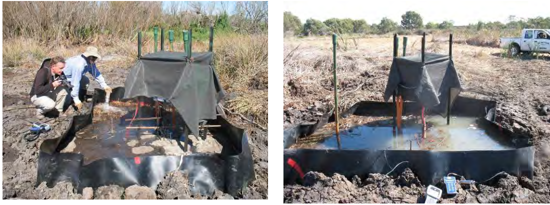
Figure 2 Reflooding experiment conducted along the River Murray (Swanport wetland) in January 2008, showing a small isolated area, which was banded using thick plastic sheeting buried to a depth of 1,5 meters, with installation of 3 piezometers and 16 redox probes (see Figure 3) connected to a data logger - being rewetted with River Murray water using a fire hose (left) and after being ponded /reflooded (right). NOTE the area only remained ponded for 1 to 3 hours due to water leakage via macro-pores.
