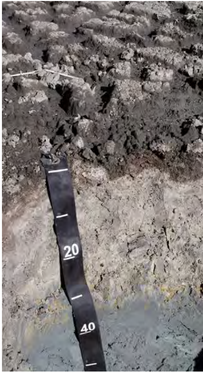
Figure 10 Acid sulfate soil (Sulfuric cracking clay soil) in the dry river bed of Boggy Creek, South Australia showing: sulfuric material (depth 0 to 38 cm with pH <4.0) with pale yellow patches or mottles of natrojarosite with minor orange-yellowish mottles comprising schwertmannite overlying dark greyish hypersulfidic material (> 38 cm). The top photograph also shows hydraulic conductivity measurements being conducted with a Guelph permeameter.
