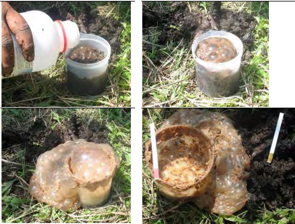
Figure 53 Photographs of the peroxide test in the field used to assess the presence of ASS (sulfidic material). Note the change in colour of the pH test strips indicating the drop in pH. Frothing and fuming is caused by the reaction of peroxide with organic matter and peroxide decomposition catalysed by metal ions. Colour changes to orange and yellow are more indicative of acid formation.
