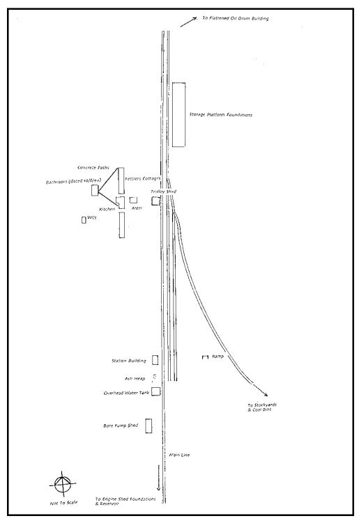
Site Plan showing significant features of the Ambinga Railway Siding Complex
