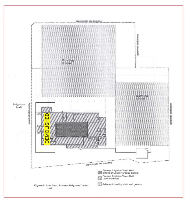
Site Plan (adapted from Flightpath Conservation Management Plan) extent of site and indicating demolished section of the building.
