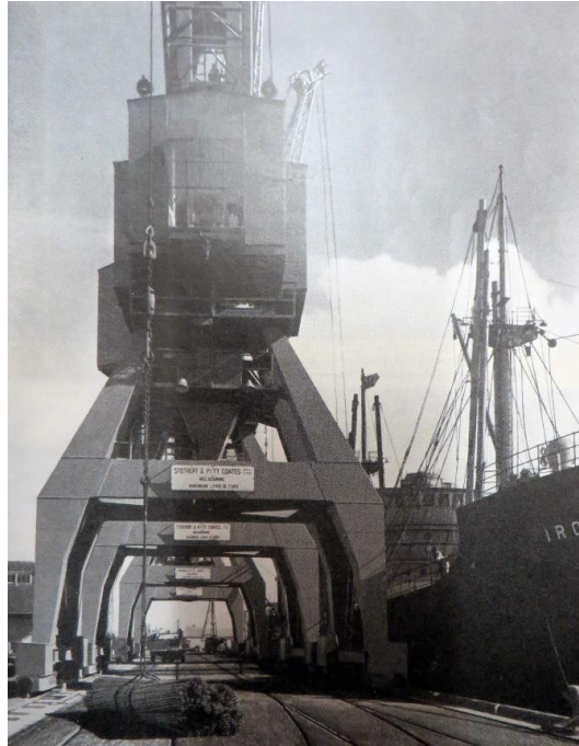
6 Ton Level Luffing Cranes, No. 2 Dock, 1958. (South Australian Harbors Board, Report of the Commissioners of the South Australian Harbors Board for the year ended 30th June 1958.)
