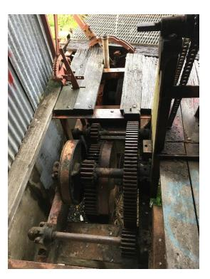
Interior workings of machinery used to turn turntable (housed in shed) Source: Heritage South Australia 19 July 2018
