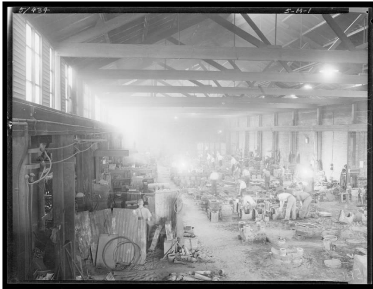
Inside the Mason Cox Foundry Southwark, c.1941, note the casting taking place directly on the sand/dirt floor.
