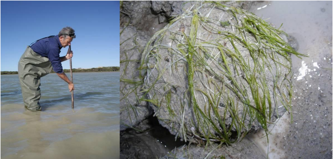
Figure 1: Colin Bailey sampling Ruppia tuberosa in the Coorong region using a corer (left) to collect a 75-mm diameter x 40-mm deep core to check for presence of Ruppia tuberosa (right). Note the turbidity of the water. (Photo courtesy Coby Mathews).
