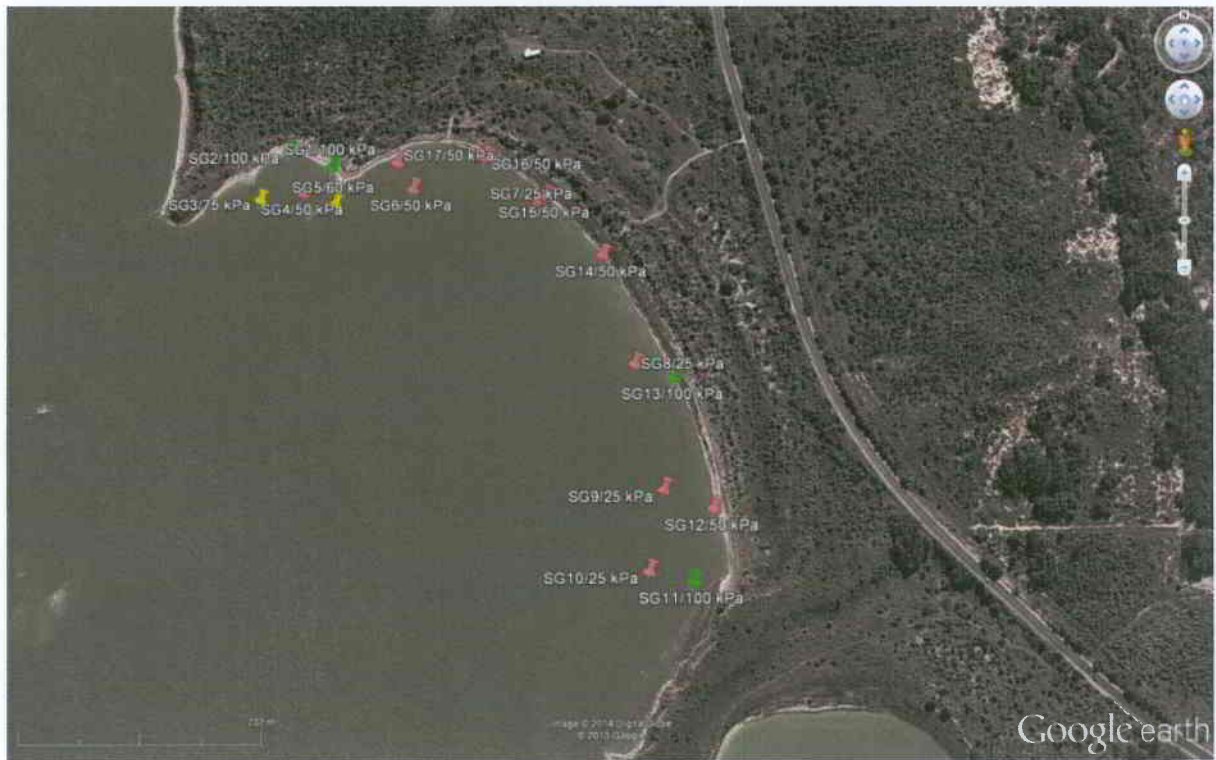
Figure 9 Sea Gull Island test locations and estimated Bearing Pressure in kPa
