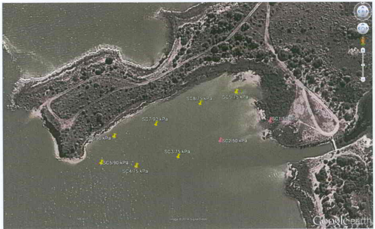
Figure 10 Salt Creek test locations and estimated Bearing Pressure in kPa
