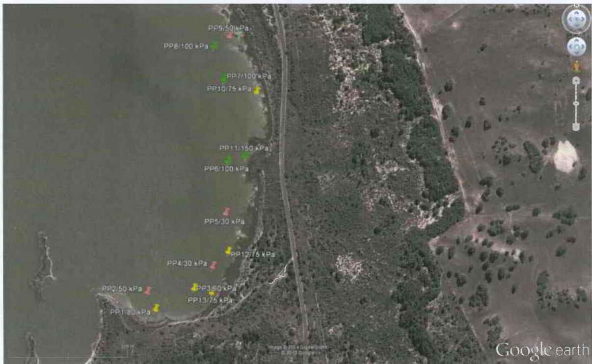
Figure 8 Policemans Point test locations and estimated Bearing Pressure in kPa
