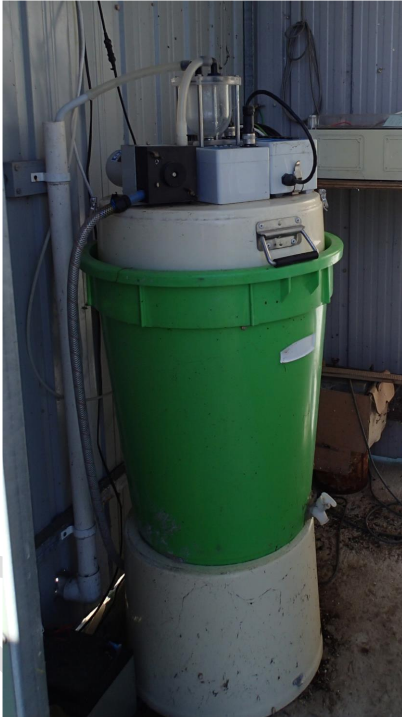
Figure 2: The composite sampler installed at the Salt Creek Flow Gauge. The peristaltic pump at the top of the bucket draws a small volume of water into the clear acrylic bowl. Once a rinse has taken place, a tap at the bottom of the acrylic bowl lets a set volume fall into the green bucket every 24 hours.
