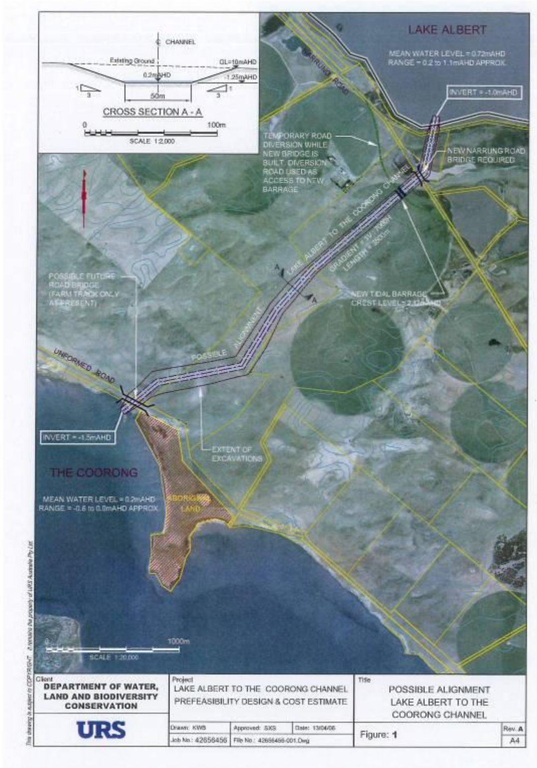
Figure 11: Potential channel design from a 2006 URS study on the Coorong Connector option
