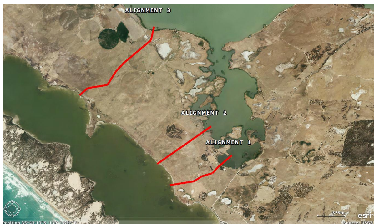
Figure 21: Possible alignments of the Coorong Connector between Lake Albert and the Coorong.
