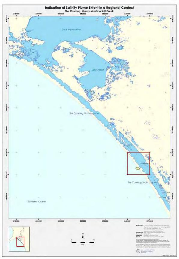
Figure 4. Indicative salinity and nutrient plume for the SLPS in a worst case scenario (The red square helps highlight the relevant area. The indicative plume of 1ppt excess salinity is in green.)
