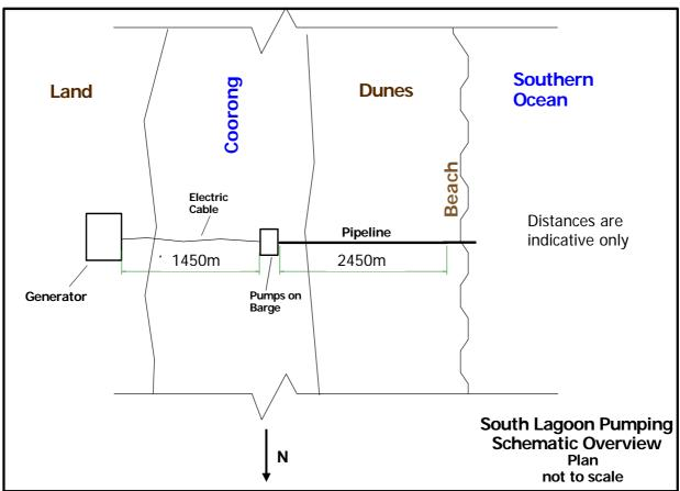
Figure 1: South Lagoon Pumping Schematic Overview (SA DWLBC).
