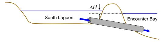
Figure 3. Schematic cross section of the South Lagoon showing a pipe connection to the sea.
