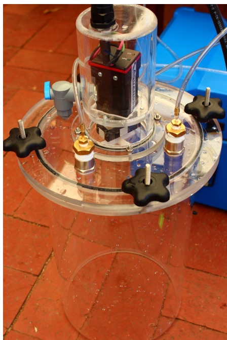
Figure 2 A photo taken prior to field testing of chamber one. Photo includes the head unit (electronic components), magnetic stirrer, gold taps, airline tubing, tie down points for weights and the series of o-rings and flanges separating each component are visible. Note there is no white collar present on this chamber.
