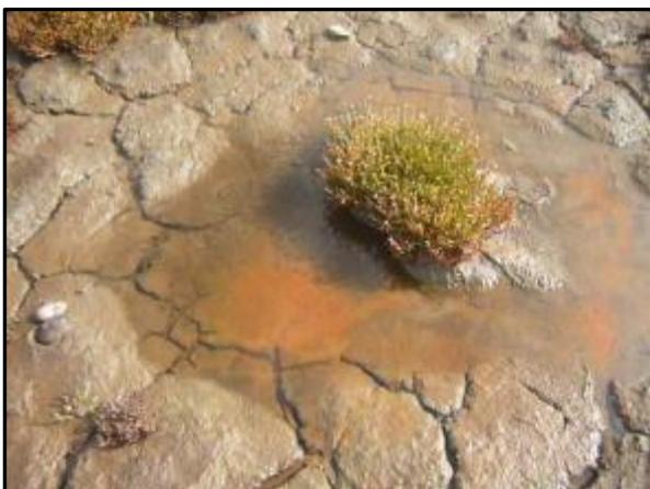
Figure 2. Characteristic red staining of sulfuric soil
