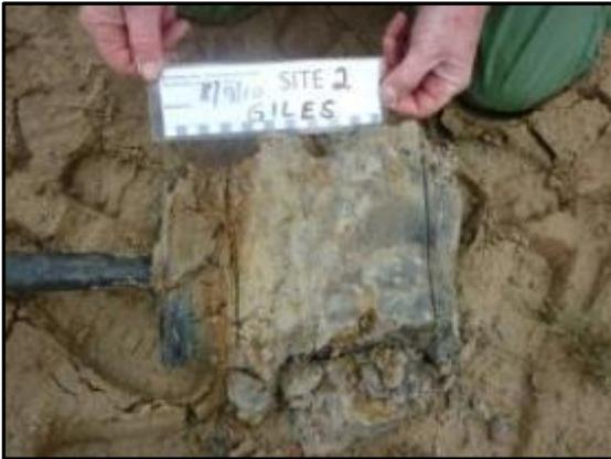
Figure 5. Original method of soil samples extraction
