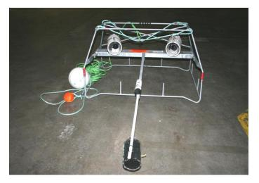
Figure 1: A stereo BRUVS unit as used in SA's marine park monitoring program
