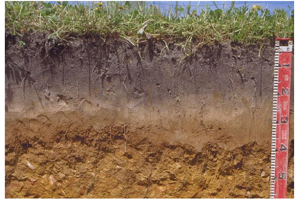
Texture can vary with depth as shown in this sand over clay soil
