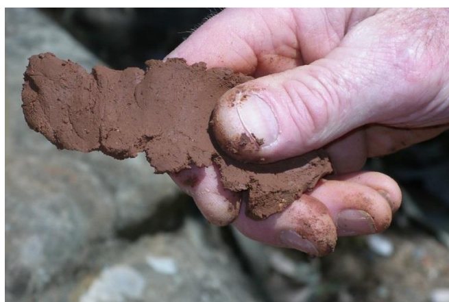
Soil texture (and an estimate of clay content) can be determined by ribboning a moistened ball of soil. The longer the ribbon, the higher the clay content is in the soil.
