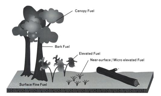
FIGURE 1 – COMPONENTS OF FUEL IN VEGETATION
