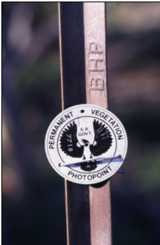
Plate 2 Standard photopoint disk attached to star dropper.
