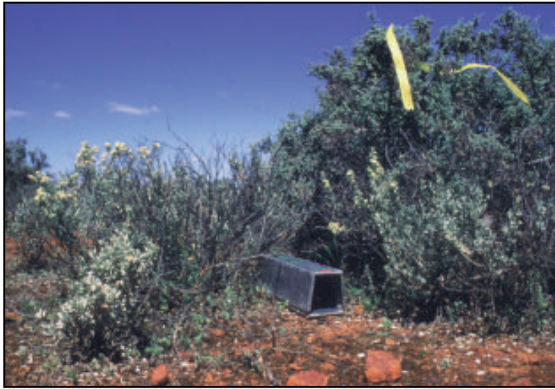
Plate 6 Elliott trap on flat, stable surface shaded by vegetation.
