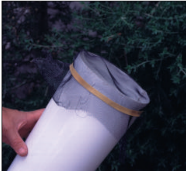
Plate 4 Poly-plastic sheet (joined with connecting strip) showing flywire bottom held in place with a rubber band.
