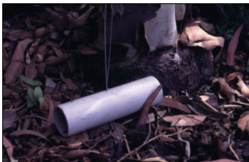
Plate 10 Hair tubes made of PVC pipe can be pegged into the ground or nailed to a tree.
