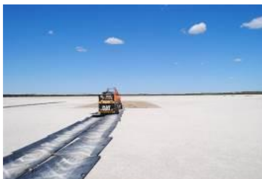
Figure 4: Excavator using track mats on lake bed at Lake Cantara, March 2013 (Photo: K. Ryan)
