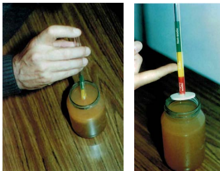
Figure A2-2. A. Left: Lowering the meter into the soil/water suspension until the white disc is no longer visible. B. Right: Reading the water level against the scale. (Source: Cox et al. 1999.)
