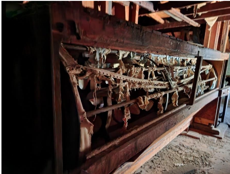
Remains of a “flour dresser” used to separate the finished flour from other grain components through gentle sifting. This was the final step in the process before the wheat was bagged.
