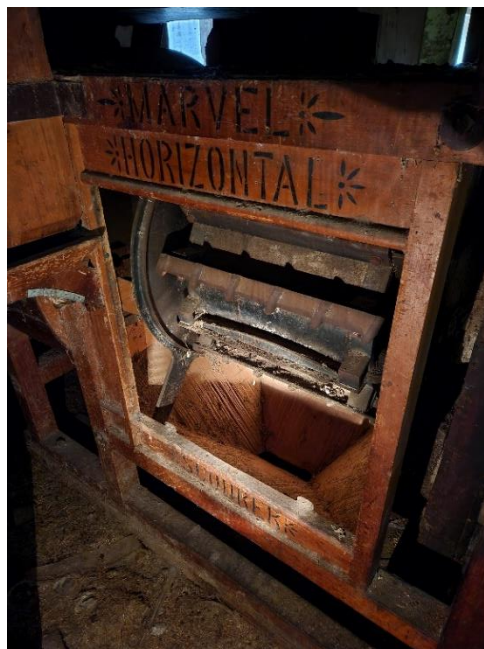
The Marvel Horizontal Wheat Scourer used to treat and clean the wheat prior to milling.
