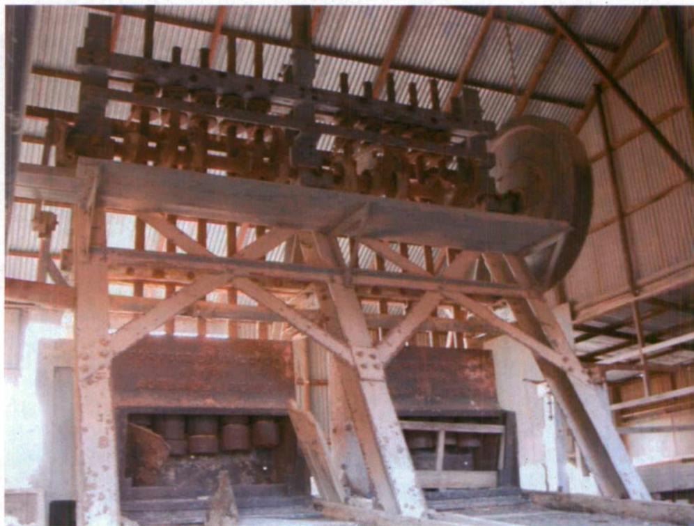
Gravity stamps, Glenloth Battery
