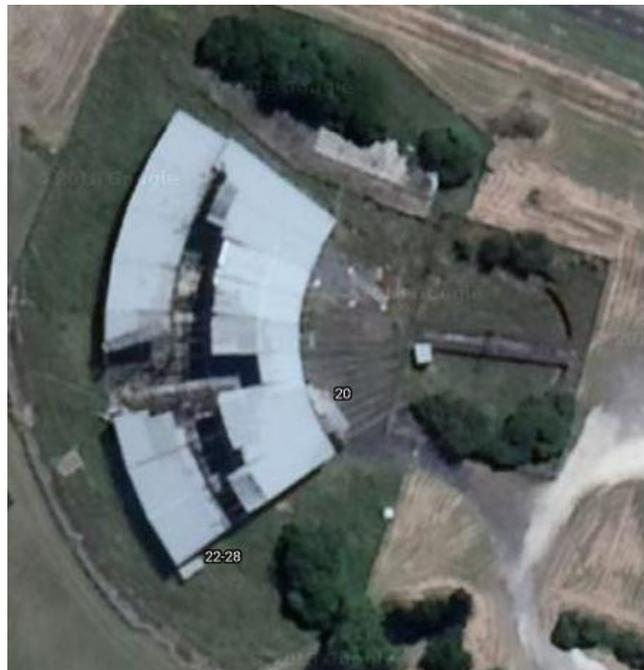
**Aerial image taken in 2018 showing the extent of loss to roof structure and rear wall.**
