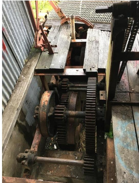
**Interior workings of machinery used to turn turntable (housed in shed)**
