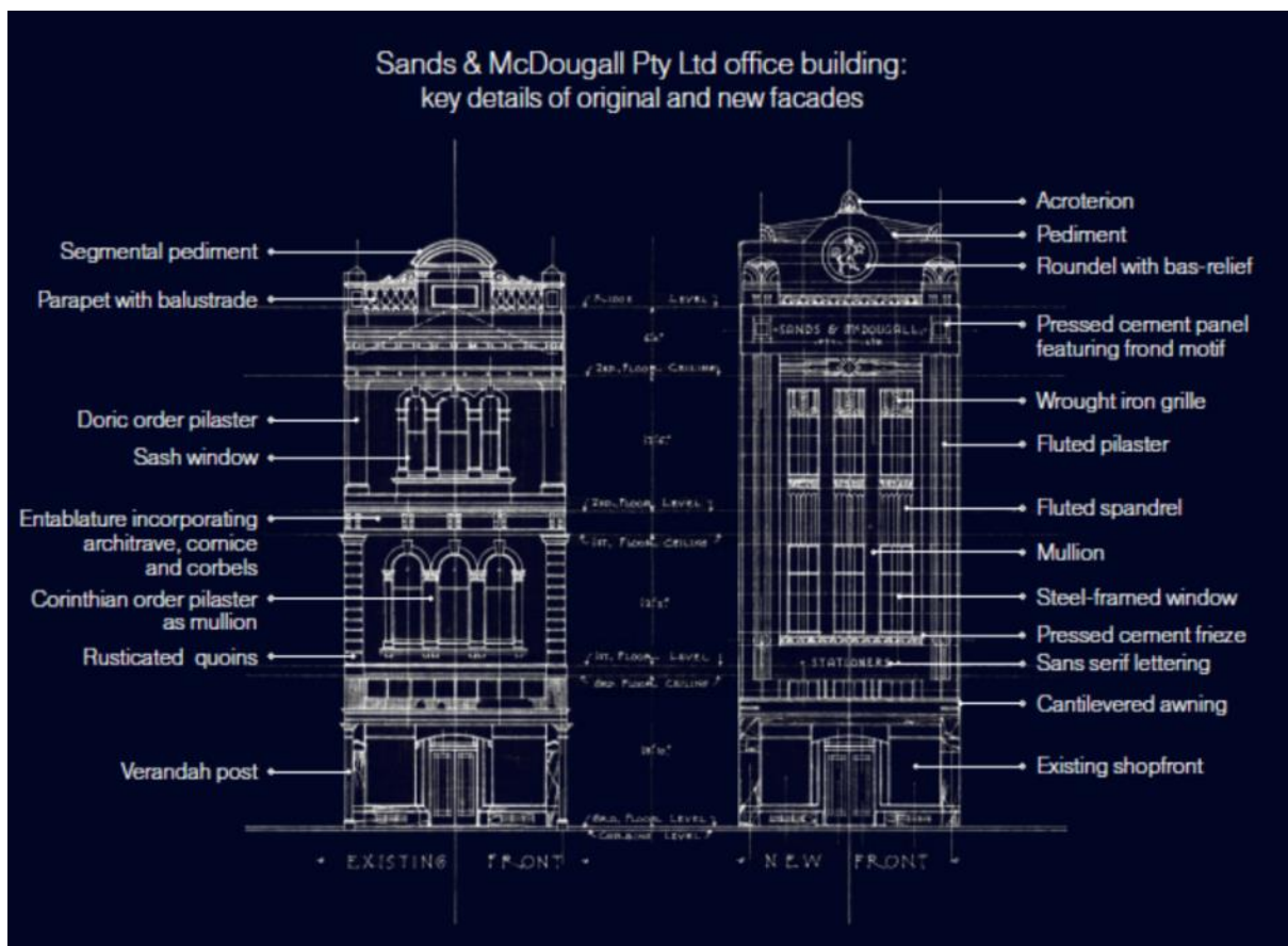
Diagram identifying the key Art Deco features of the Sands & McDougall Building. Note where the diagram states a pressed cement frieze, it is made from copper or a copper alloy.
