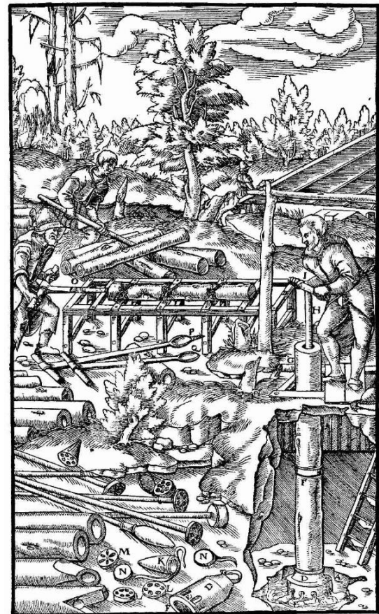
A—SUMP. B—PIPES. C—FLOORING. D—TRUNK. E—PERFORATIONS OF TRUNK. F—VALVE. G—SPOUT. H—PISTON-ROD. I—HAND-BAR OF PISTON. K—SHOE. L—DISC WITH ROUND OPENINGS. M—DISC WITH OVAL OPENINGS. N—COVER. O—THIS MAN IS BORING LOGS AND MAKING THEM INTO PIPES. P—BORER WITH AUGER. Q—WIDER BORER.
