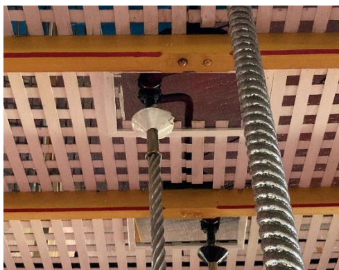
Typical connections between crankshaft and barley-twist horse rods, with oil cups.
