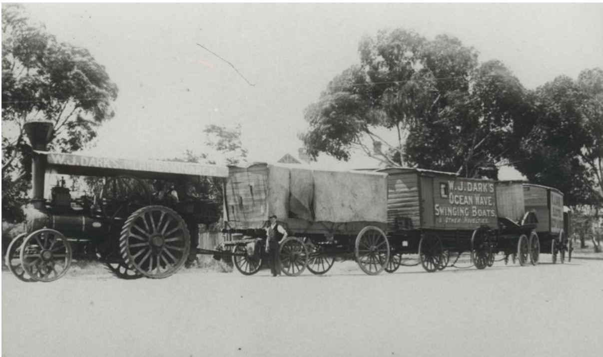
W. J. Dark's road train at Willunga, 1907. The third wagon behind the traction engine is the centre truck of Dark's Electric Merry-Go-Round (note hinged centre pole/flue collapsed for transport), while the fourth wagon contains disassembled carousel components including sweeps, rounding boards, scenic panels, rods and horses.
