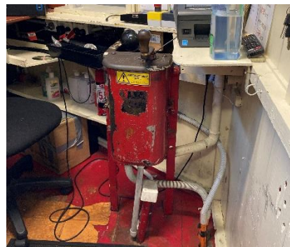
Carousel controller (ex MTT tram controller).
