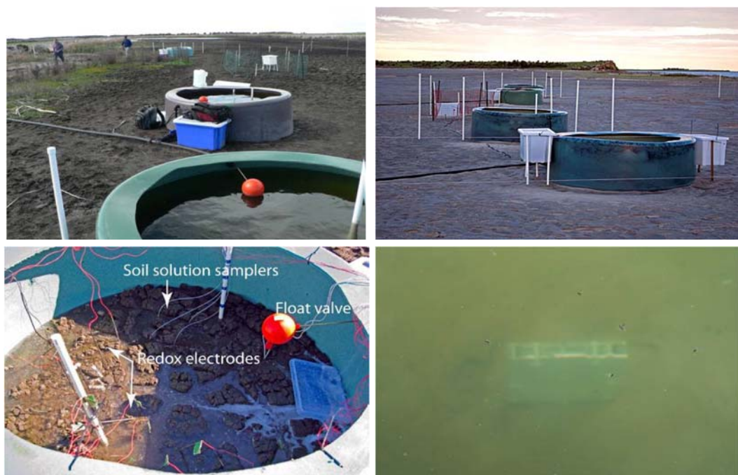
Figure 10. Mesocosm infrastructure at Boggy Creek (top left) and Point Sturt (top right). Instrumentation included piezometers and soil solution samplers (lower left) and peepers (lower right).
