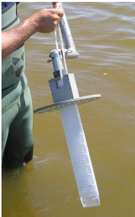
Figure 5-2. Photo showing lower end of specialised peeper installation apparatus with peeper ready to be deployed.
