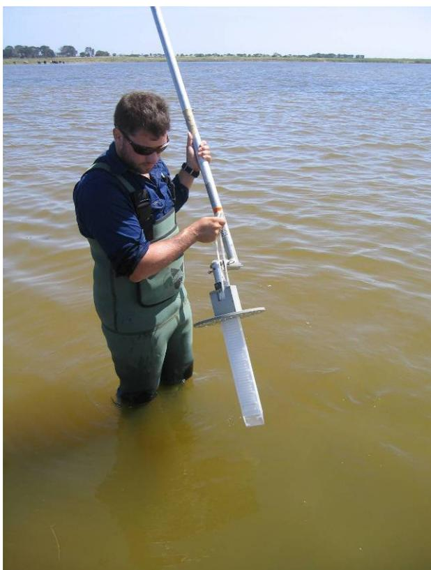
Figure 2-1. Soil pore water sampler (white plastic with 36 cells) carefully pushed into the sediment to a set depth.
