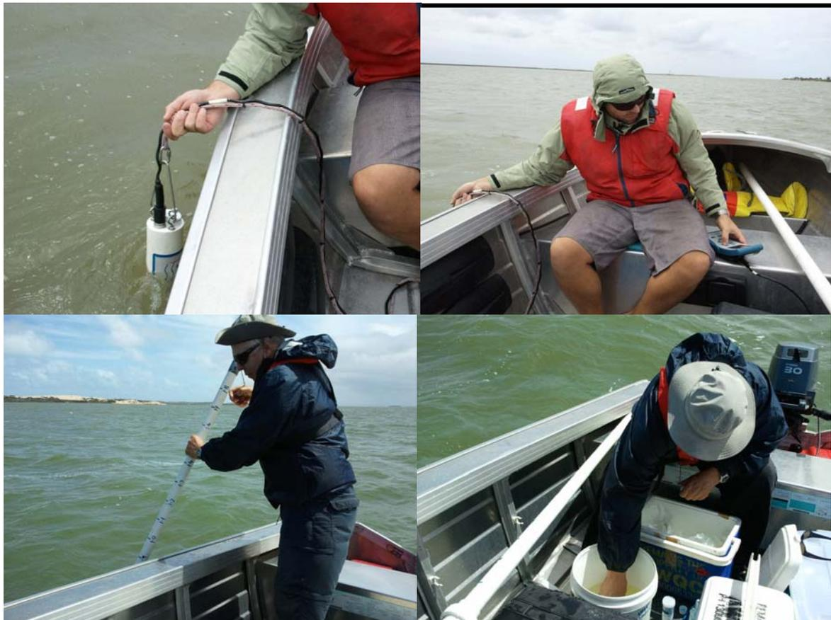
Figure 3. Photos of field work for microalgae in the Coorong. Top left: lowering multi-probe through the water column. Top right: recording readings from multi-probe. Bottom left: collecting integrated water samples. Bottom right: collecting microalgal samples.
