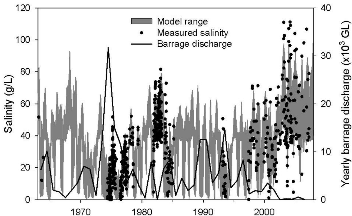
**Figure 1** Observed salinity and barrage flows in the Coorong North Lagoon and modelled salinity range from hydrodynamic modelling. Image provided by Ian Webster, CSIRO.
