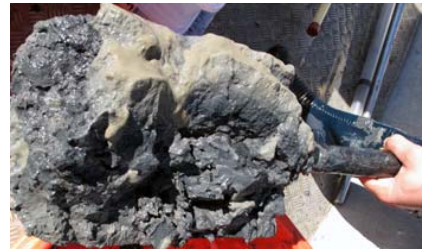
Soils being described, placed in chip-tray and mixed prior to placing in sample jars.
