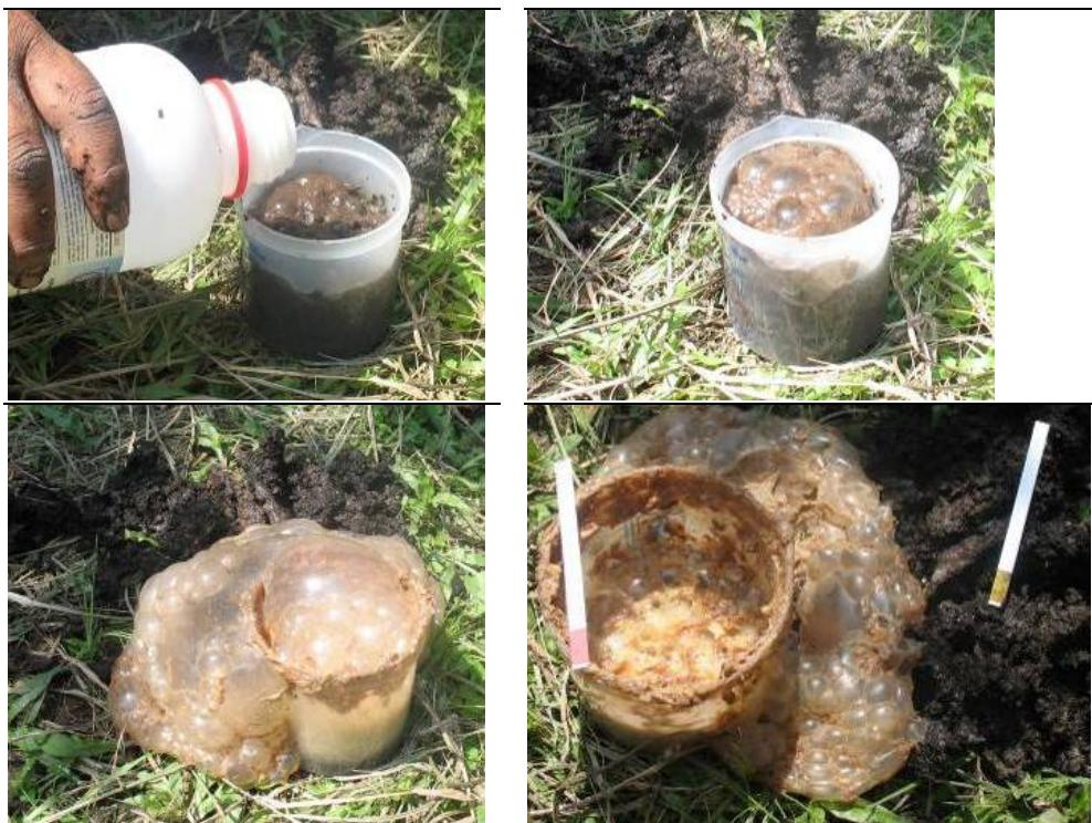
Figure 53. Photographs of the peroxide test in the field used to assess the presence of ASS (sulfidic material). Note the change in colour of the pH test strips indicating the drop in pH. Frothing and fuming is caused by the reaction of peroxide with organic matter and peroxide decomposition catalysed by metal ions. Colour changes to orange and yellow are more indicative of acid formation.
