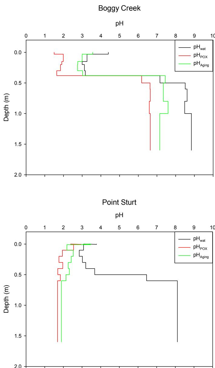
**Figure 12** Soil pH profiles. If  $\text{pH}_{\text{wat}} < 4$  the soil material is sulfuric, if  $\text{pH}_{\text{POX}}$  or  $\text{pH}_{\text{Aging}} < 4$  the material is hypersulfidic
