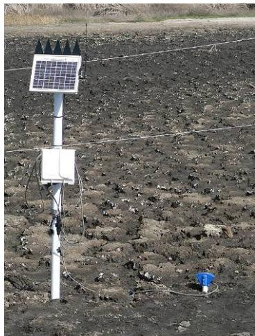
Figure 5 Sentek probe and telemetry station
