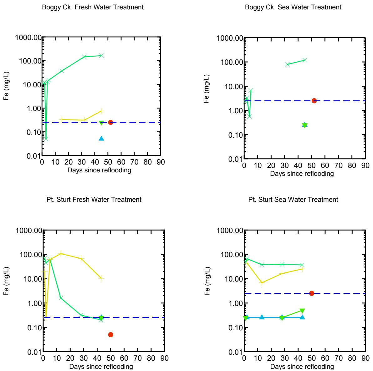
**Figure 29** Time series for total iron concentration. Surface Water =  $\textcolor{red}{\circ}$ , Pore Water:  $\textcolor{green}{\times}$  = 0.2 m bgl,  $\textcolor{yellow}{+}$  = 0.5 m bgl,  $\textcolor{blue}{\Delta}$  = 1.0 m bgl,  $\textcolor{green}{\nabla}$  = 1.5 m bgl. The blue dashed line represents the highest instrumental detection limit for the particular parameter-matrix combination; in some cases this may be lower depending on sample ionic strength (salinity).
