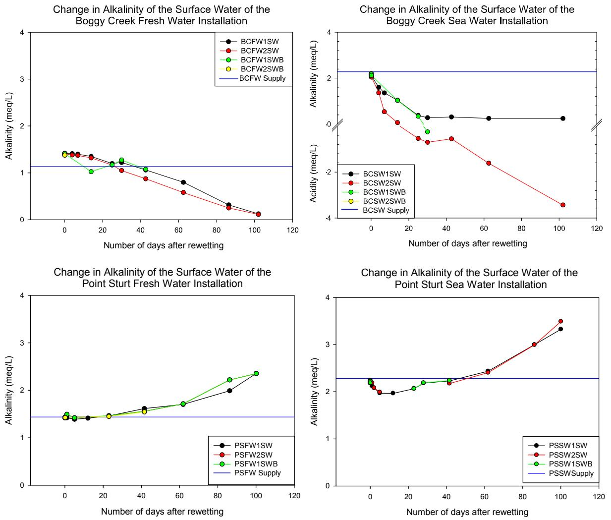
Figure 24 Time series for surface water alkalinity.
