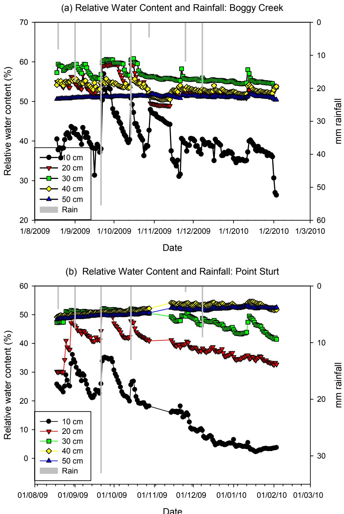
Figure 18 Relative water content and rainfall. Relative water contents are uncalibrated raw data and only trends and relative change can be inferred, for example this means that in plot (b) ~50% may represent field capacity and that comparison between sites cannot be made.
