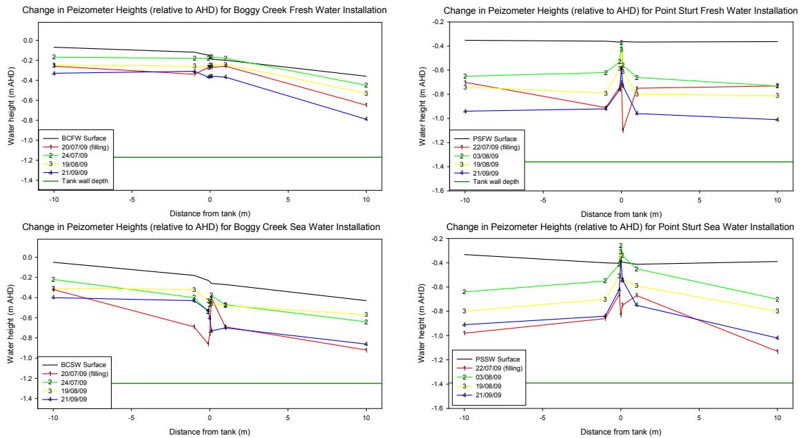
**Figure 15 Piezometer heights along transects. Negative distance value means towards the bank or shore line from the installations, whereas positive distance value means towards the channel or lake edge. The black line indicates the ground elevation of the piezometer. The dark green line indicates the depth of the tank wall**
