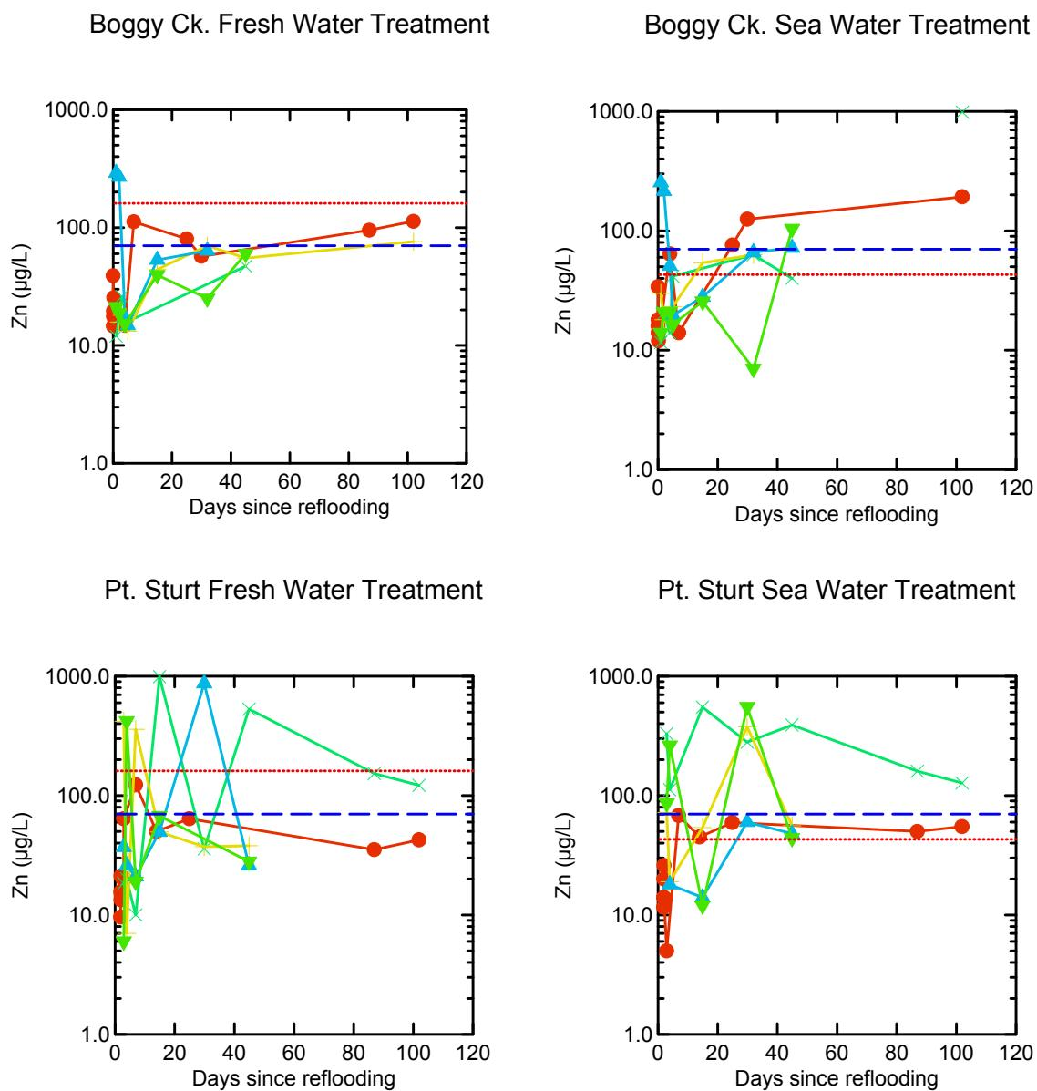
**Figure 47 Zinc.** Surface Water = O, Pore Water:  $\times$  = 0.2 m bgl, + = 0.5 m bgl,  $\Delta$  = 1.0 m bgl,  $\nabla$  = 1.5 m bgl. The blue dashed line represents the detection. The red dotted line represents the relevant ANZECC and ARMCANZ WQ guideline trigger value for toxicants at the 80% protection level. Analyses were undertaken on  $<0.22\text{ }\mu\text{m}$  filtered samples. Toxicant fresh water values have been corrected for hardness (extremely hard water).
