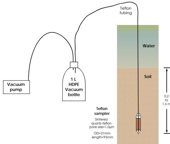
Figure 6 Diagrammatic representation of Teflon™ sampler deployment
