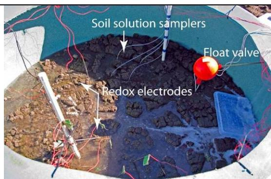
Figure 8 Mesocosm showing monitoring devices during flooding
