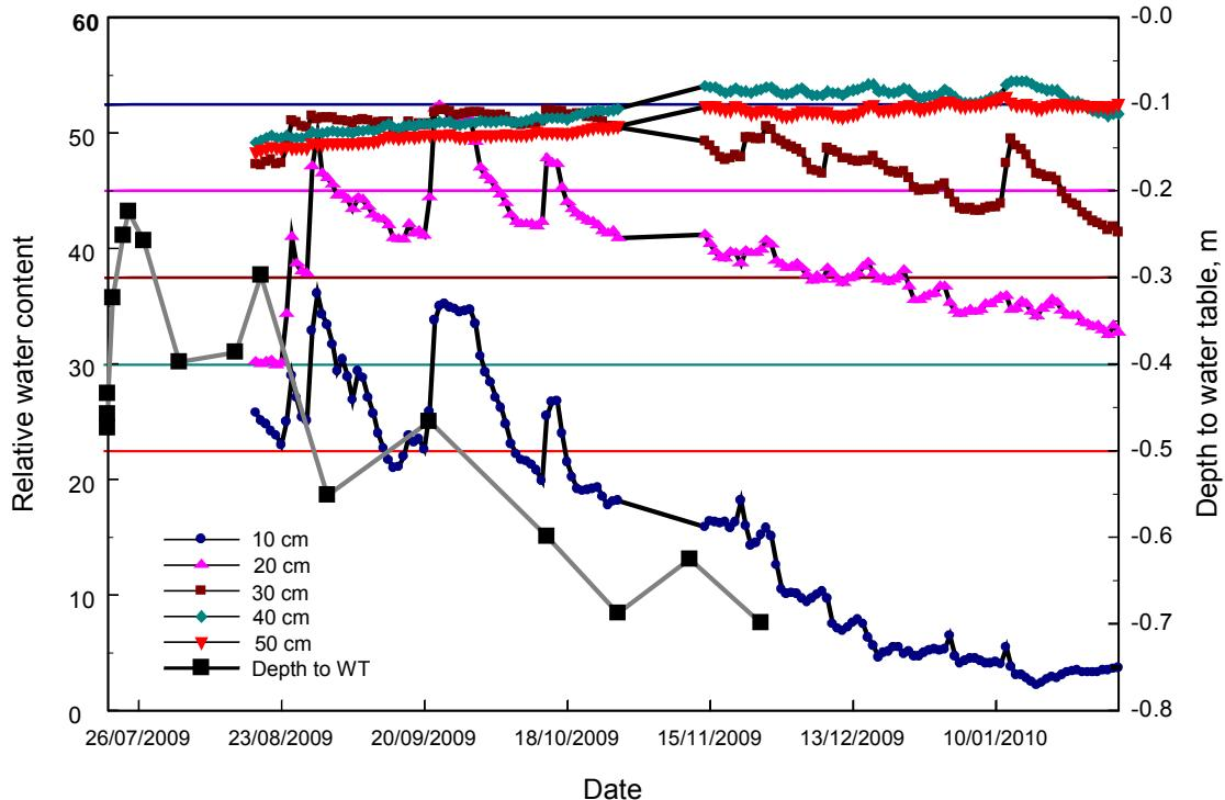
Figure 17 Relative water contents and depth to water table. Horizontal lines represent sensor depths and are colour keyed to corresponding relative water content scatter plot. Relative water contents are uncalibrated raw data and only trends and relative change can be inferred, for example this means that in plot (b) ~50% may represent field capacity.
