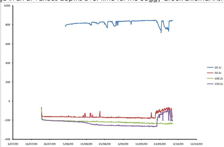
**Figure 19** Time series for soil redox potential at the Boggy Ck. site. The tanks were filled on 21/7/09.
