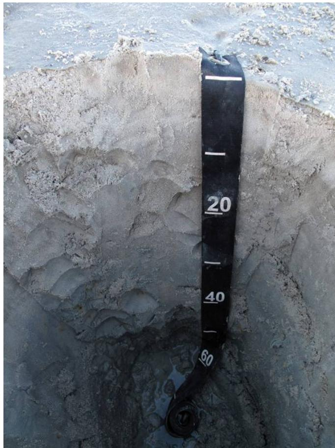
**Figure 11 Acid sulfate soil (Sulfuric soil) on the dry bed of Lake Alexandrina on the South's property, Point Sturt peninsula, South Australia showing: sulfuric material (depth 0 to 50 cm with pH <4.0) with hypersulfidic material (> 50 cm) occurring below the current water table**
