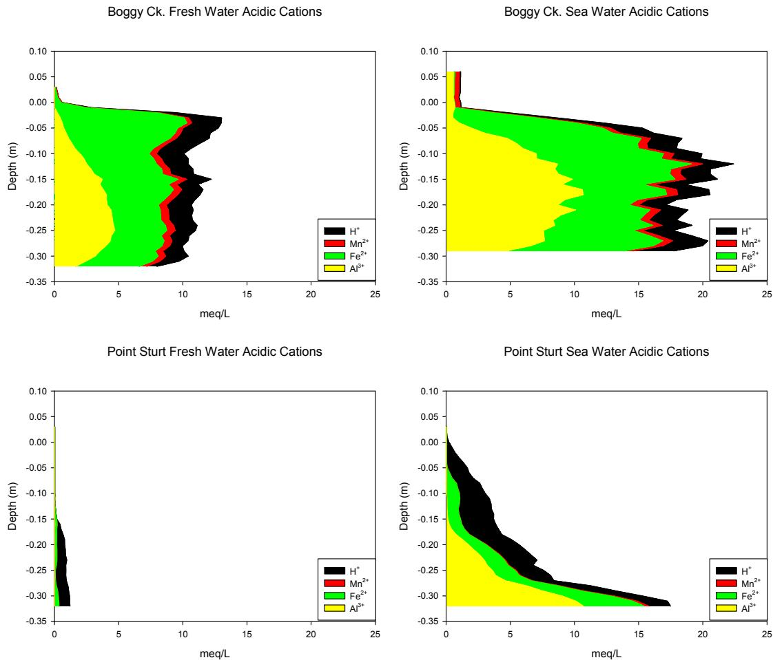
**Figure 30** Soil profile of total acidic cations from dialysis chamber samplers deployed for the period 18/08/09 to 03/09/09. The profiles show the contribution of each cation. The horizontal width of the coloured band represents the concentration of that species. The distance from the vertical axis to the right hand edge of the band represents the total of acid cations for all species included in that horizontal slice.
