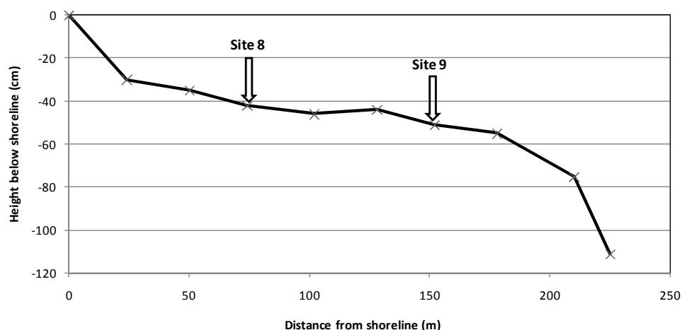
Figure 5-14. Shoreline cross-section at Site 8 and 9.
