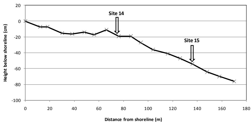
Figure 5-23. Shoreline cross-section at Site 14 and 15.
