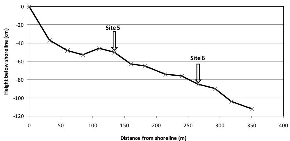
Figure 5-9. Shoreline cross-section at Site 5 and 6.
