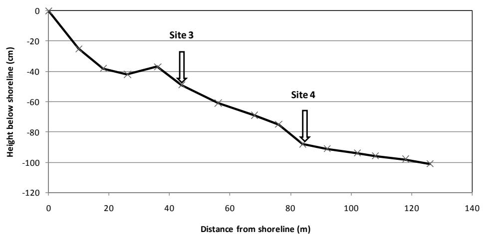
Figure 5-6. Shoreline cross-section at Site 3 and 4.
