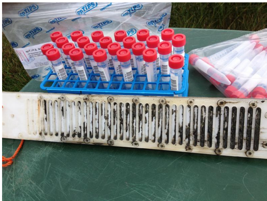
Figure 3 A peeper following retrieval, ready to be rinsed and the filling solution in the chambers extracted.
