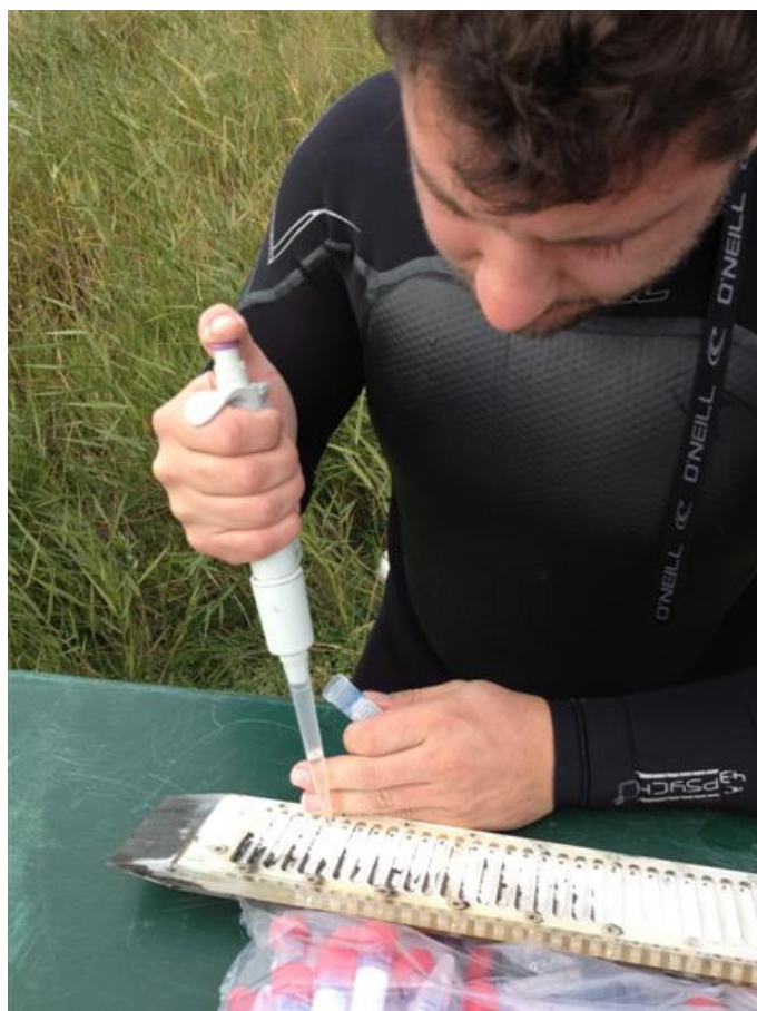
Figure 4 Extracting the pore water from the chambers of the peeper.
