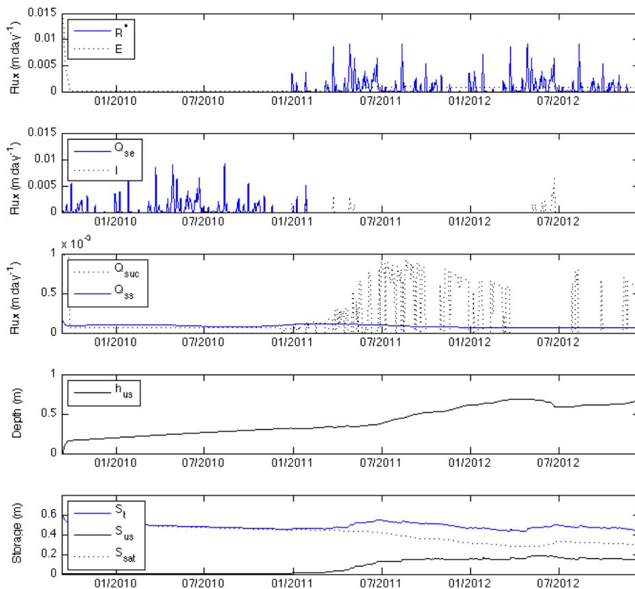
Figure 7.34: Hydrology fluxes in Lake Alexandrina drawdown simulation for a boundary sand cell. Refer to Figure 4.2 for symbol definitions and the hydrological conceptual model.
