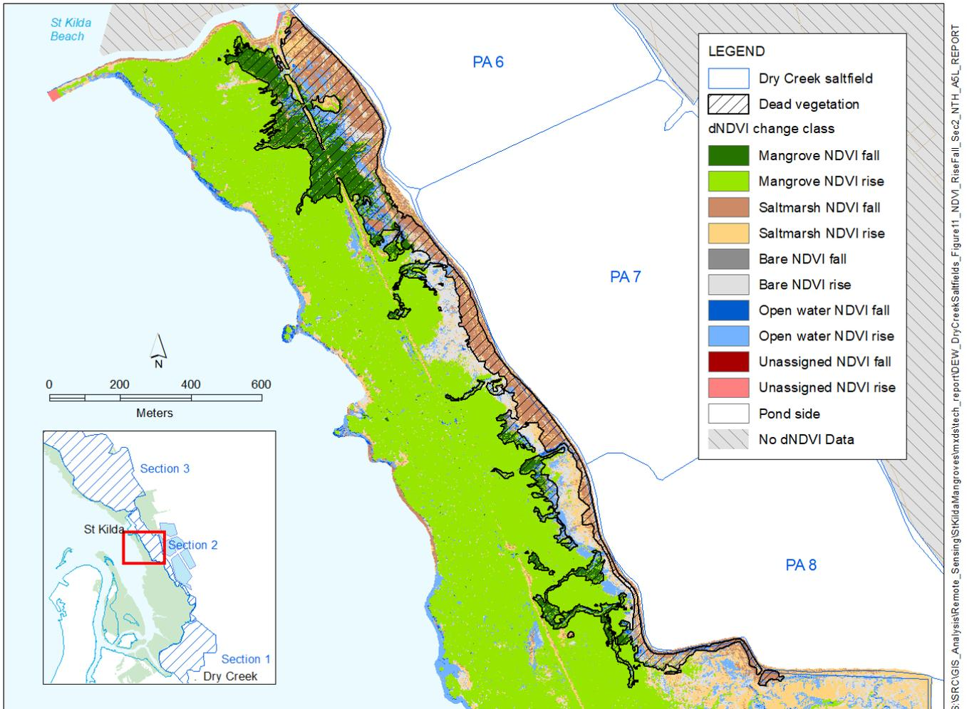
**Figure 13**  $dNDVI$  thresholded hyperspectral vegetation/ land cover classes overlaid with manual mapping in northern parts of section 2.
