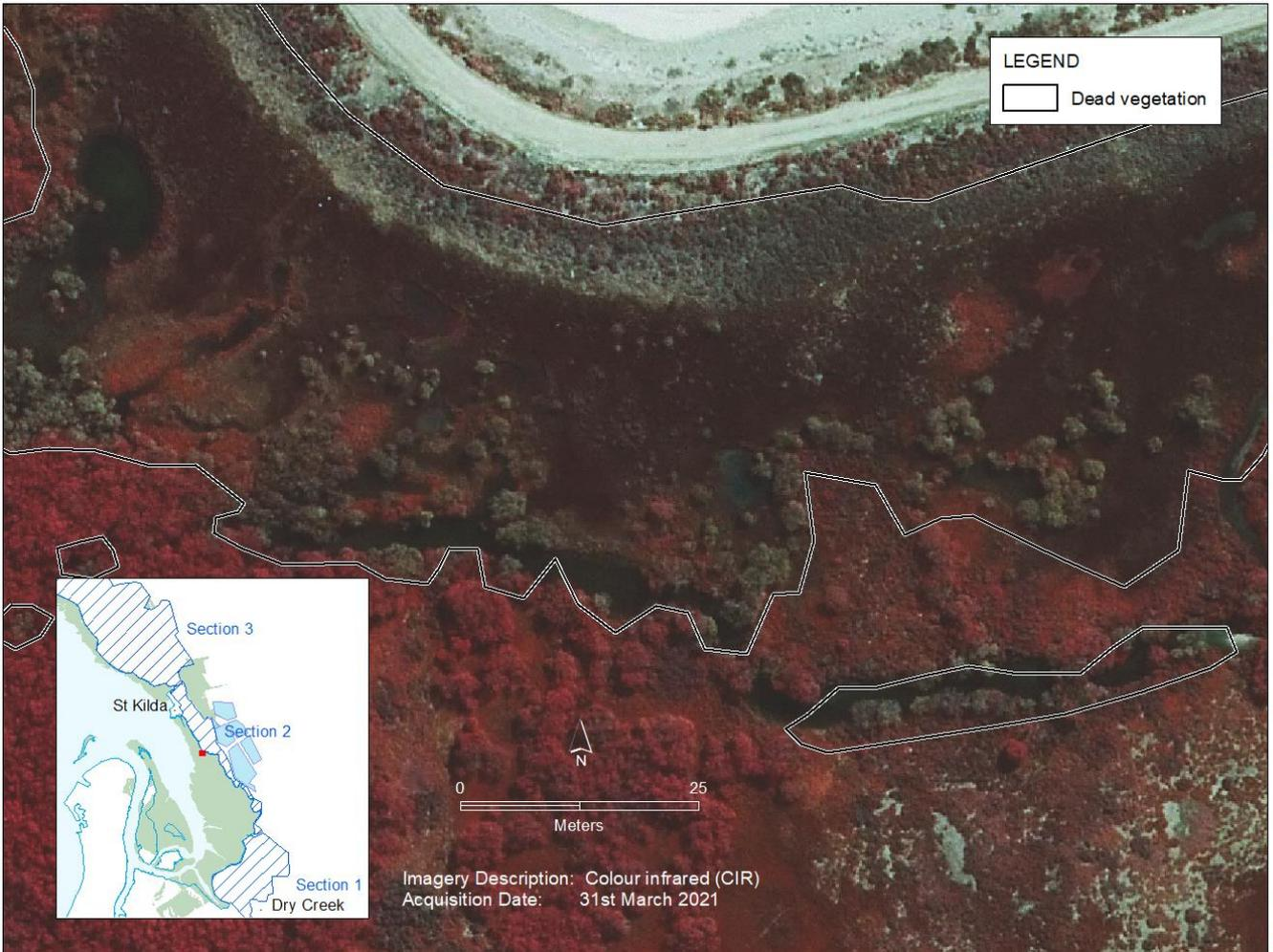
**Figure 3 shows use of false colour (infra-red) image to delineate dead vegetation at screen scale of 1:800. Red tones are healthy vegetation, grey tones are dead. Note mangrove trees, water in creeks and light coloured bare ground are visible whereas smaller saltmarsh species are less distinct in terms of form and colour.**
