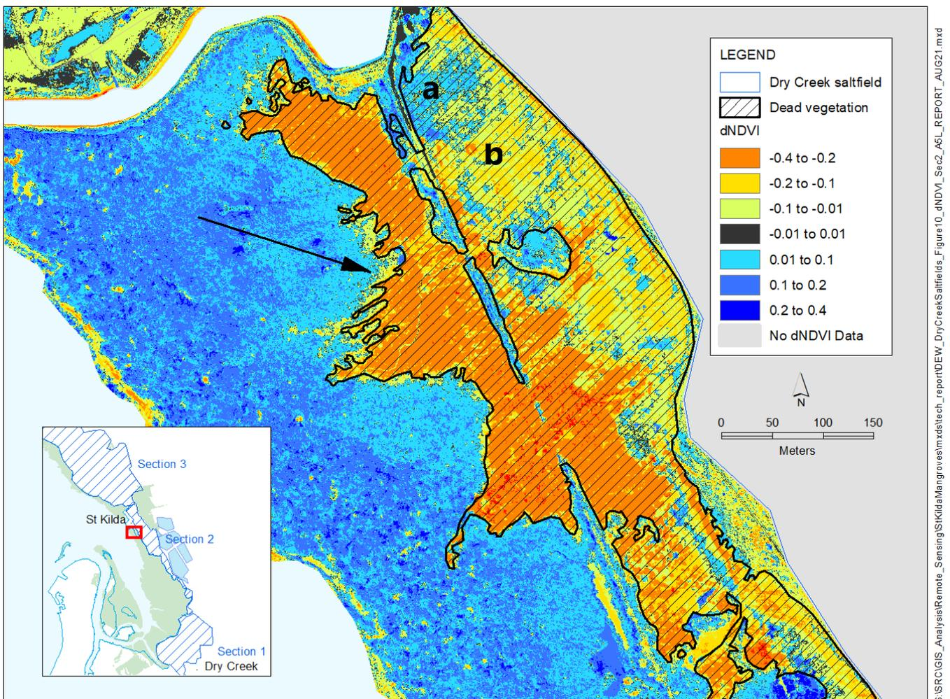
**Figure 12 NDVI change mapping (dNDVI) between 2018 and 2021 showing alignment of manual mapping (black outline) with reduced NDVI (orange and yellow tones), plus the conundrum of both a rise in NDVI (blue tones at a) as well as a fall in NDVI (yellow tones at b) within the manually mapped dead saltmarsh.**
