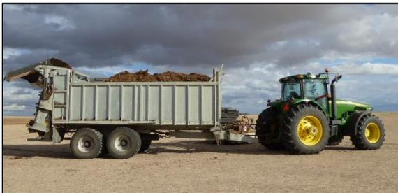
*Manure applied across bare soil using a spreader. Some issues with fine particles lost in the wind, larger manure clods (fresh manure) are preferable for stabilising the soil surface.*
