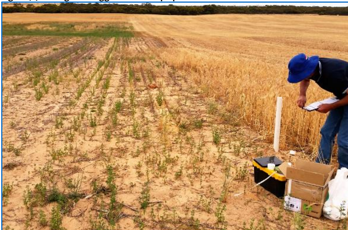
Figure 74. Fitting data logger to mid-slope piezometer
