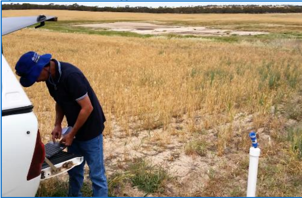
Figure 38. Piezometer data logger installation at bottom, soak site
