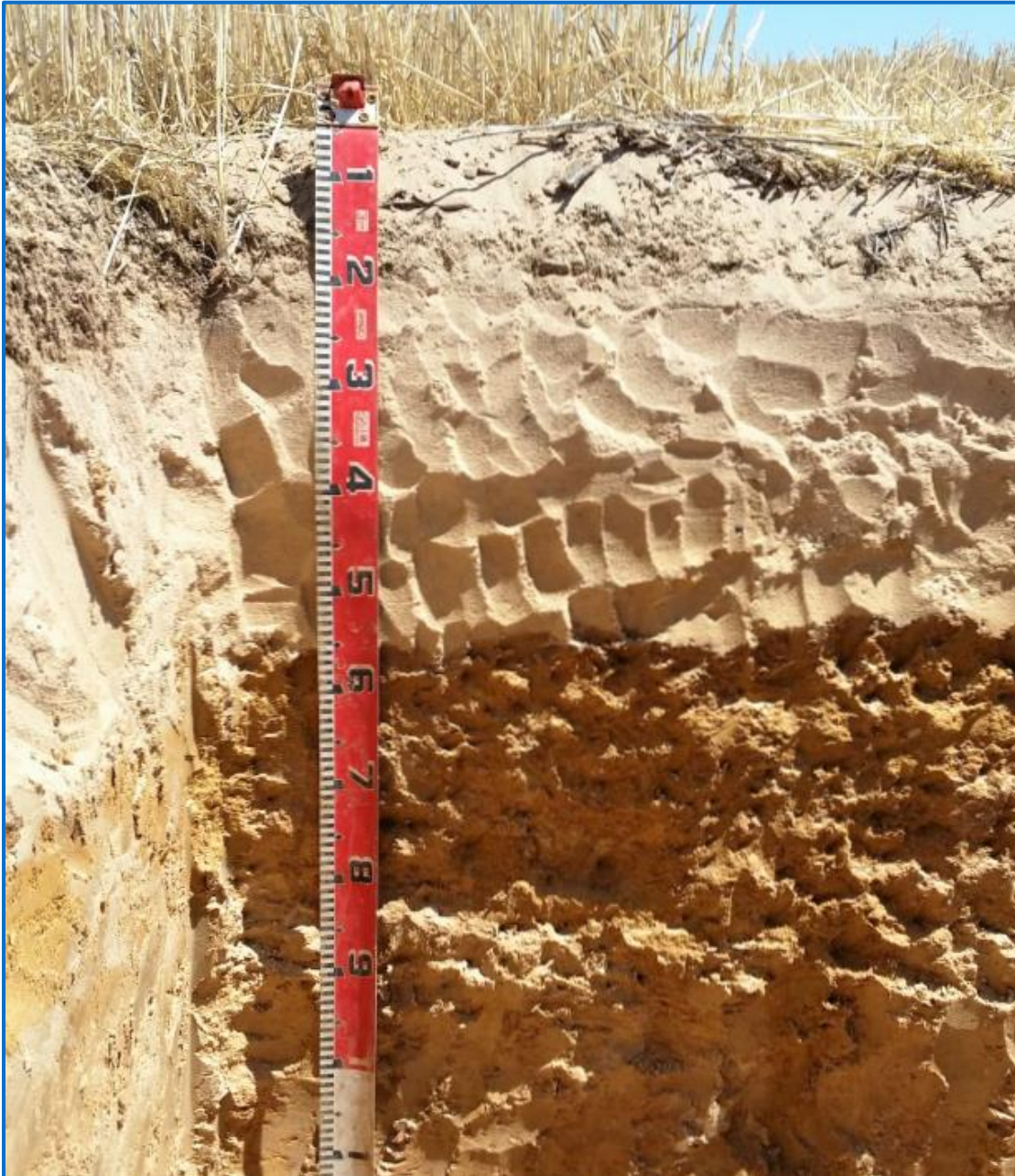
Figure 31. New soil pit with sand over clay at 60cm just above trial site
