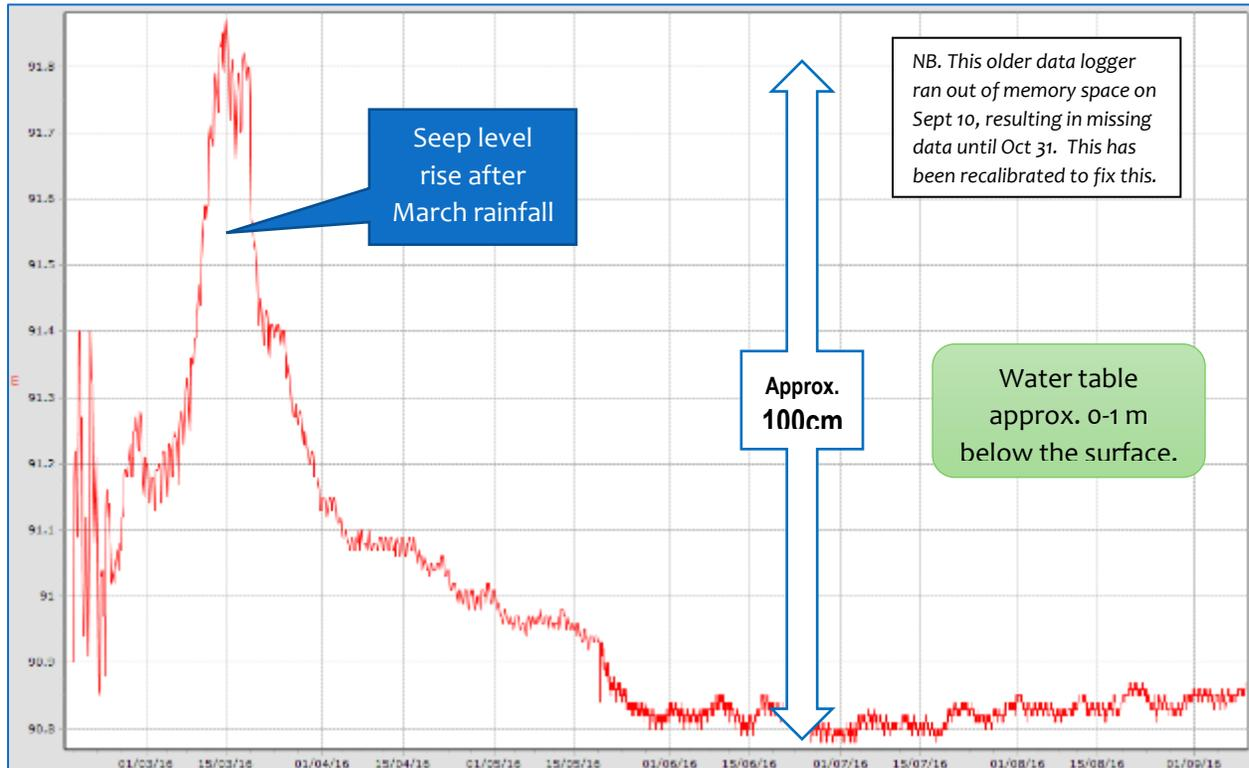
**Fig 7. Groundwater level for Piezometer 9, high southern seep, Nov - Dec 2016**
