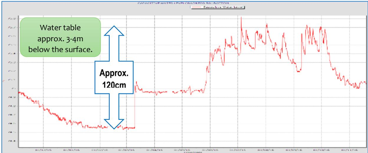
**Fig 32. Piezometer B02 readings from the top of non-wetting sandy rise, Nov 2015 - Nov 2016**
