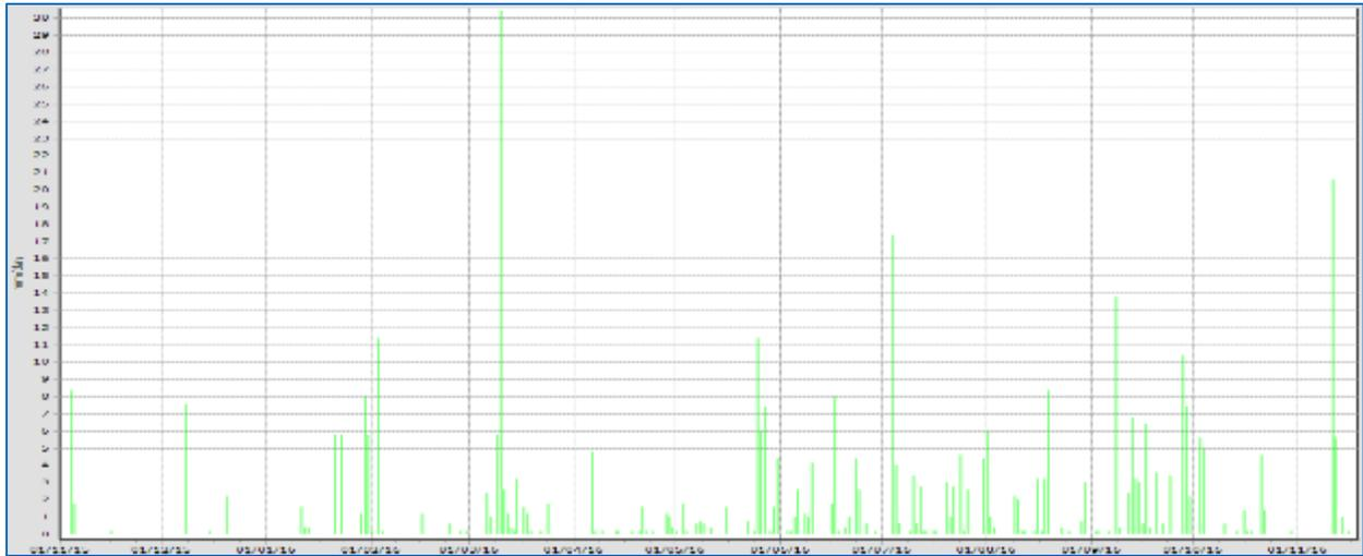
**Fig 31. Piezometer B01 readings for Bottom soak area, Nov 2015 - Nov 2016**
