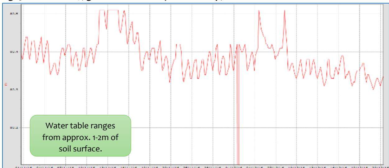
**Fig 14. Piezometer 6, groundwater level for eastern fenceline, March - Aug 2016**
