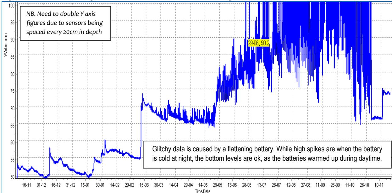
**Fig 62. Lucerne system moisture probe readings, Nov 2015 – Nov 2016**
