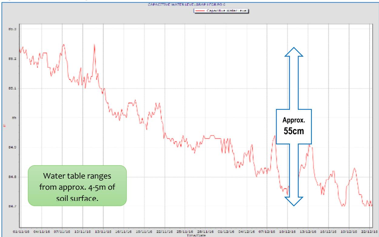
**Fig 16. Piezometer 5, moisture readings for southern fence line, Nov - Dec 2016**
