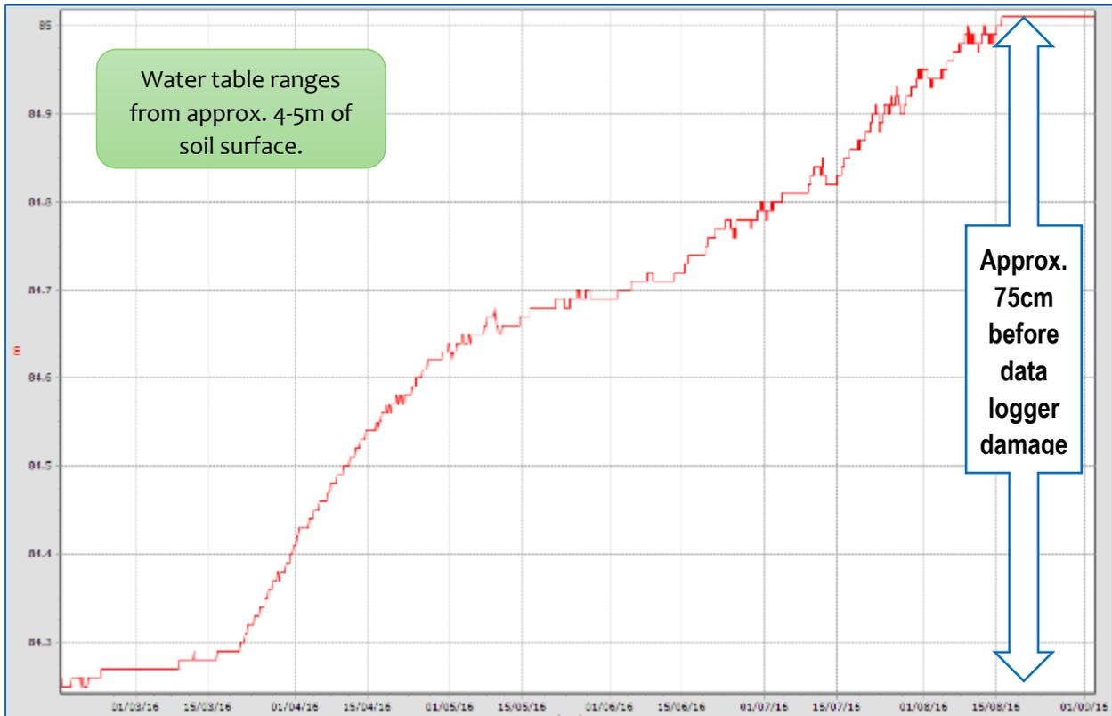
**Fig 15. Piezometer 6, groundwater level for eastern fenceline, Nov - Dec 2016**
