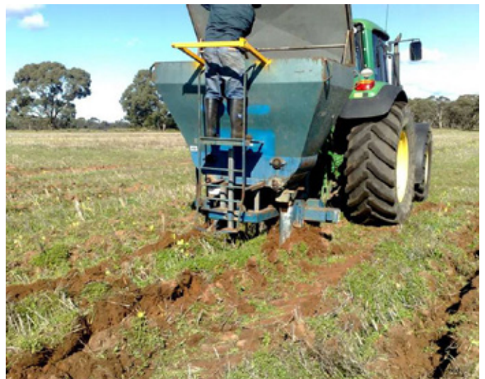
The subsoil manuring machine applying treatments in 2015.
