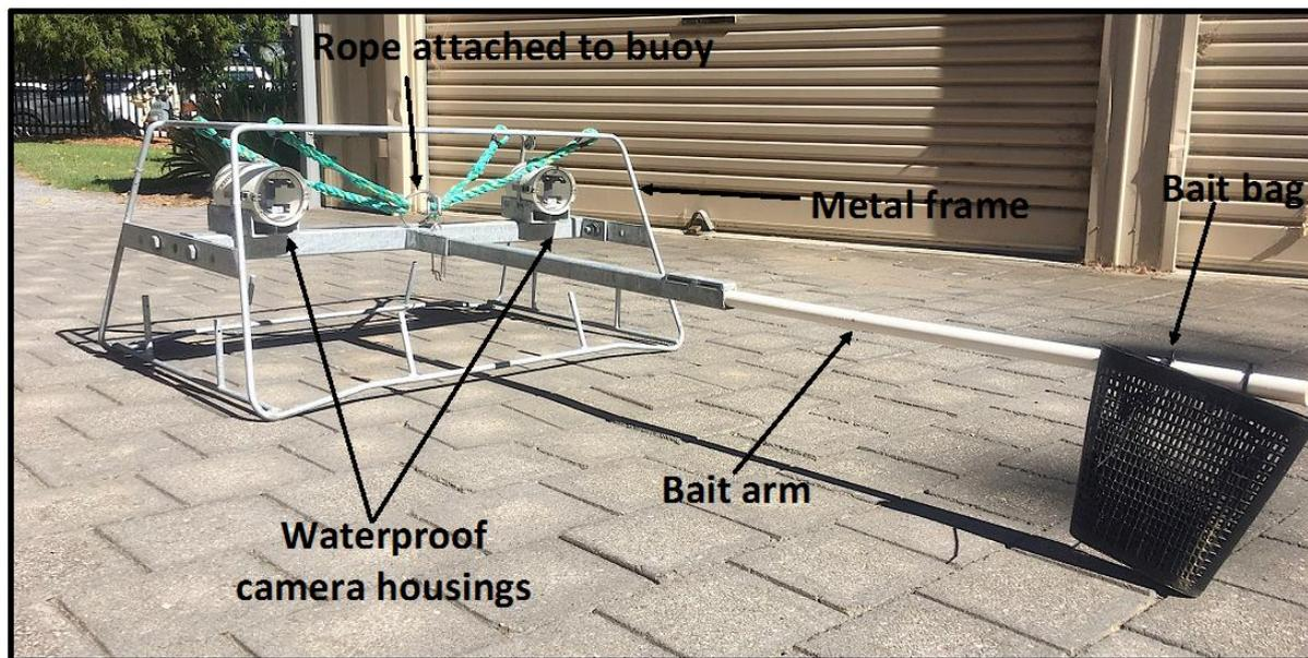
**Figure 3.** BRUV unit. Frame constructed of aluminium; bait arm was constructed of PVC pipe and bait pouch gutter mesh; ropes were connected to a metal ring on one end and the other end was connected to a buoy which allowed the unit to be deployed and retrieved remotely; GoPro video cameras were mounted inside the underwater housings.
