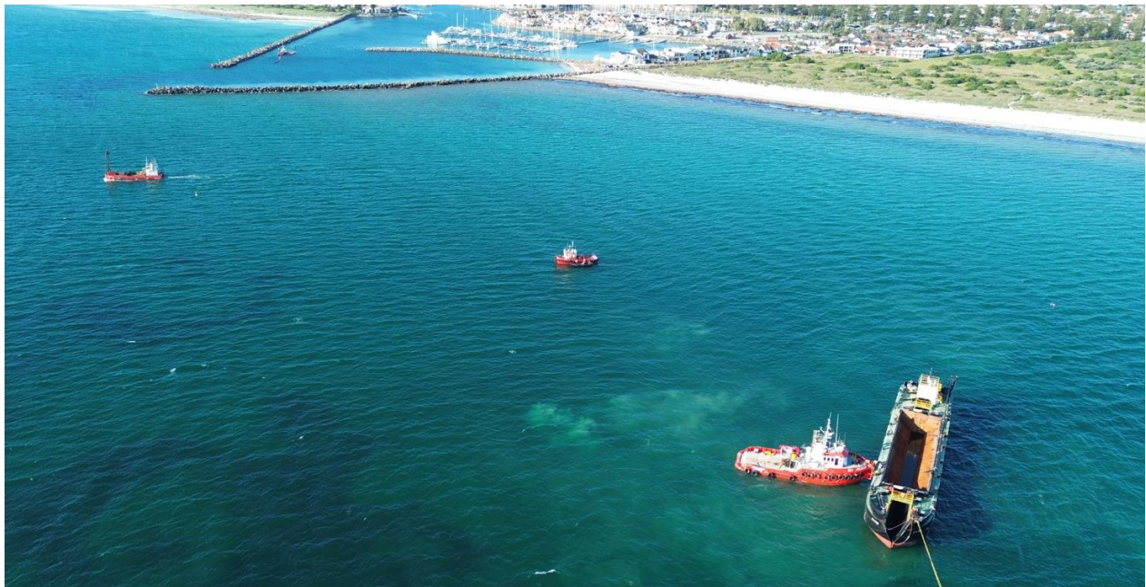
Figure 1. Dredging at sand source area SBA1 with CSD Kingston (left), anchor barge (middle) and split hopper barge WH762 supported by Sea Pelican tug (right)
