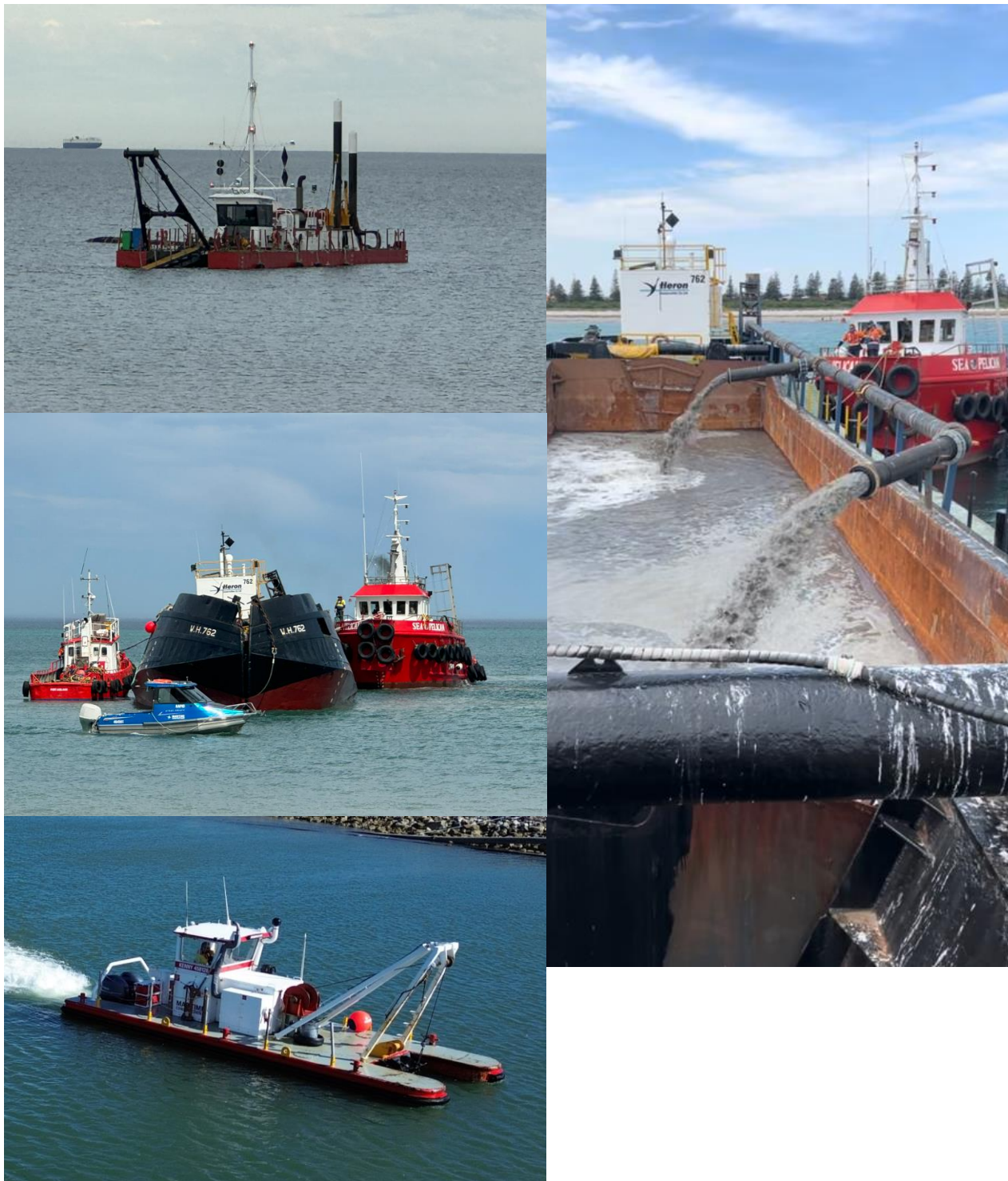
Figure 3. Key Marine Plant – CSD Kingston (top left); Chapman, Rapid, WH762 & Sea Pelican (middle), anchor barge Kenny (bottom left) and filling hopper barge WH762 (right)
