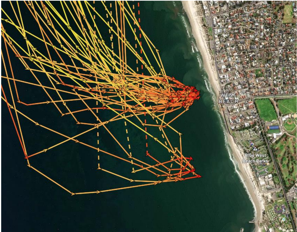
Figure 7. SHB nearshore sand placement at West Beach SPA1 North and Rehandling Area (3 – 21 October)
